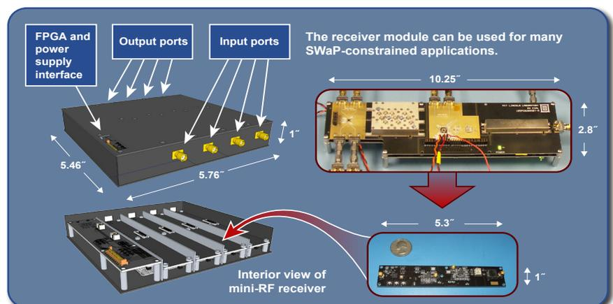
**Figure 1. The four-channel mini-RF receiver occupies a single 6U VME card by replacing larger, low-yielding materials with SiGe semiconductors. For comparison, a commercial two-channel RF receiver uses four 6U VME cards.**
