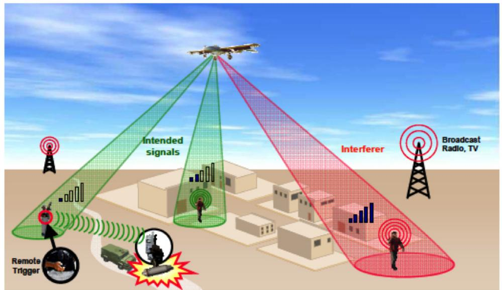
**Figure 2.** A scenario illustrating the Lincoln Laboratory mini-RF receiver system mounted on an aircraft as well as the sources of desired signals (shown in green) and sources of interfering signals (shown in red).
