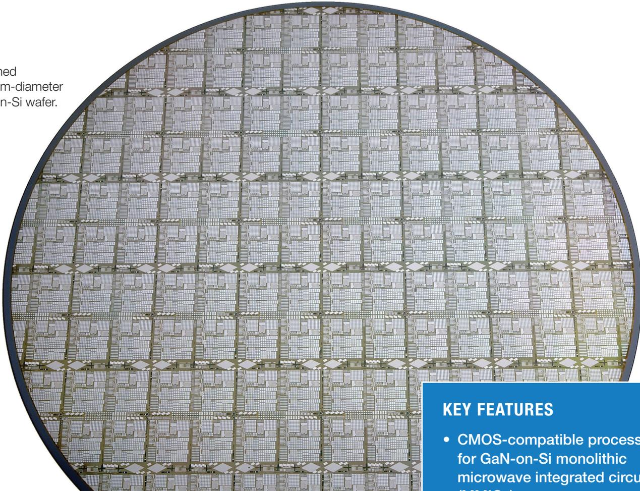
Lincoln Laboratory developed fully Si CMOS-compatible technologies for GaN MMICs on 200-mm-diameter Si wafers. Measured  $f_T$  and  $f_{max}$  are in the 50 and 90 GHz range, respectively, for GaN high-electron-mobility transistors (HEMTs) with 120-nm gate length on Si substrates. We are applying wafer-scale 3D integration technology to the heterogeneous integration of GaN MMICs and Si CMOS circuits for high-performance RF modules.
