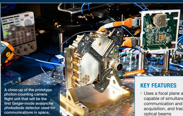
The photon-counting camera utilizes Lincoln Laboratory's novel array of Geiger-mode avalanche photodiodes integrated with a custom integrated circuit to enable two-way optical communications from deep space. This deep-space optical communication system's ability to provide high-data-rate transmissions could expand the possibilities for human and robotic deep-space exploration.
