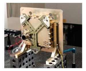
The photon-counting camera. The Y-shaped bracket mounts the camera to the rest of the deepspace optical communication system. The baffle (tube shape) on the Y protects the camera's optical path from stray light. Support electronics are in a chassis behind the Y bracket, and the metal plate behind the camera is a radiator to cool the camera.
