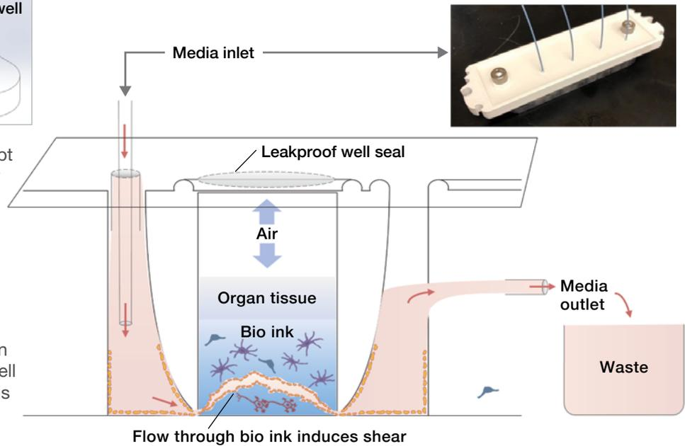
This illustration shows the concept of operation of the neurovascular unit that enables co-culturing of tissues for the study of the blood-brain barrier. Liquid media is injected into each well. As the media pumps through the bio ink, it creates the shear flow that promotes vascular tissue development. The organ tissue on top of the bio ink and air in the well are sealed in, and excess media is drawn off as waste.
