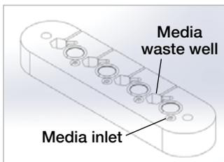
Fluidic ribbon connector enables liquid-tight, easy on-and-off connections to the vasculature
