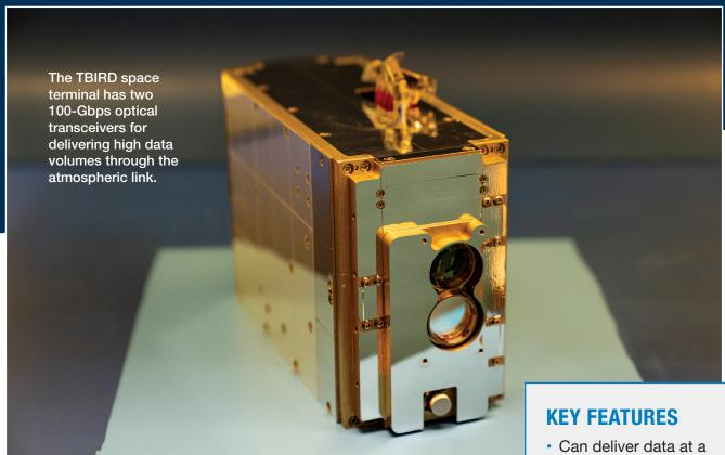
Lincoln Laboratory in collaboration with NASA has developed optical communication technology to enable the transmittal of data from low Earth-orbiting satellites to ground stations at the revolutionary rate of 200 gigabits per second. This fast, error-free transfer of extremely high volumes of data may transform the operations and missions of scientific, commercial, and defense satellites.
