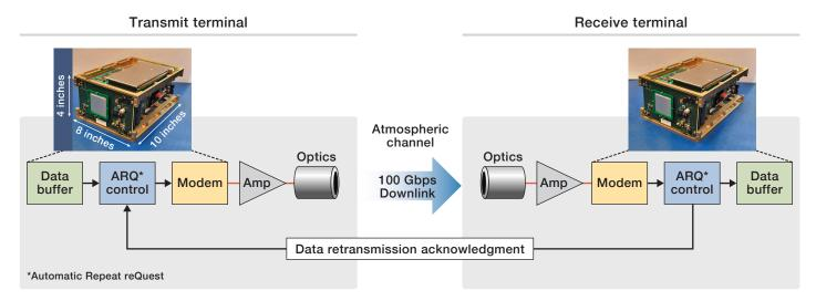
The TBIRD system is an augmented modem that can achieve reliable communication through challenging free-space channels when paired with a telescope and pointing system. The ARQ control can request the retransmission of data packets that were not successfully received. This redundancy reinforces a transmission of an error-free message. The transmit and receive platform could be space, ground, or airborne.
