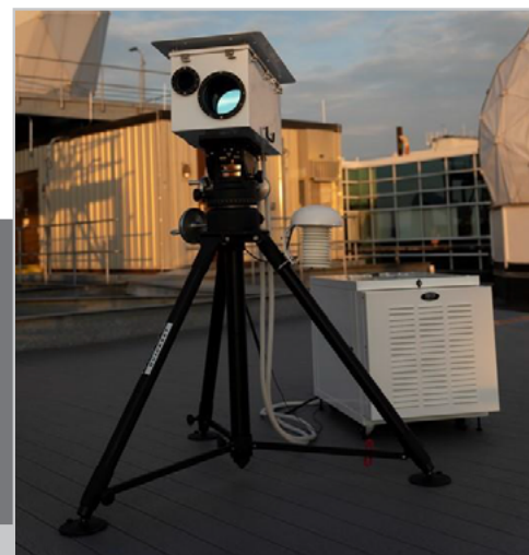
Above, a ruggedized sensor is mounted on a base so it can be set up unattended to monitor a region of airspace.
