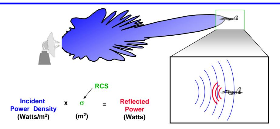
Radar Cross Section (RCS, or s) is the <u>effective</u> crosssectional area of the target as seen by the radar
