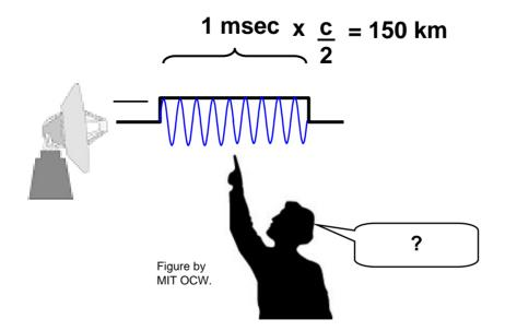
Solution: Use pulse with changing frequency and signal process using "matched filter"
