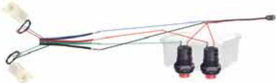
Connect the battery and determine which motor is connected to the left and right switches
