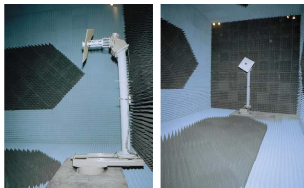
FIGURE 14. Lincoln Laboratory’s millimeter-wave anechoic chamber is an ideal location to test the EBG’s capability of reducing or eliminating propagation between nearby monopole antennas. The electromagnetic shielding and interior wall configurations reduce the noise levels.
