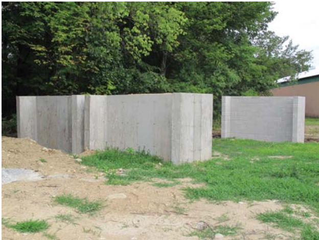
FIGURE 11. The "test range" for through-wall measurements shows the 10 cm and 20 cm thick, solid concrete walls on the left and the cinder-block wall on the right.
