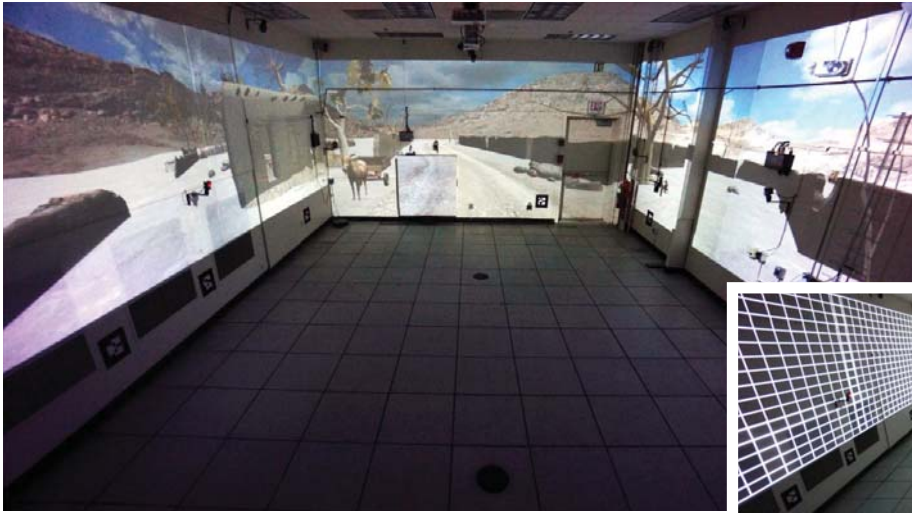
The Lincoln Laboratory Interactive Virtual Environment (L-Live) superimposes the virtual world on three sidewalls in the 3D infrared tracking theater (large photo) for a 270° displayable area (inset).
