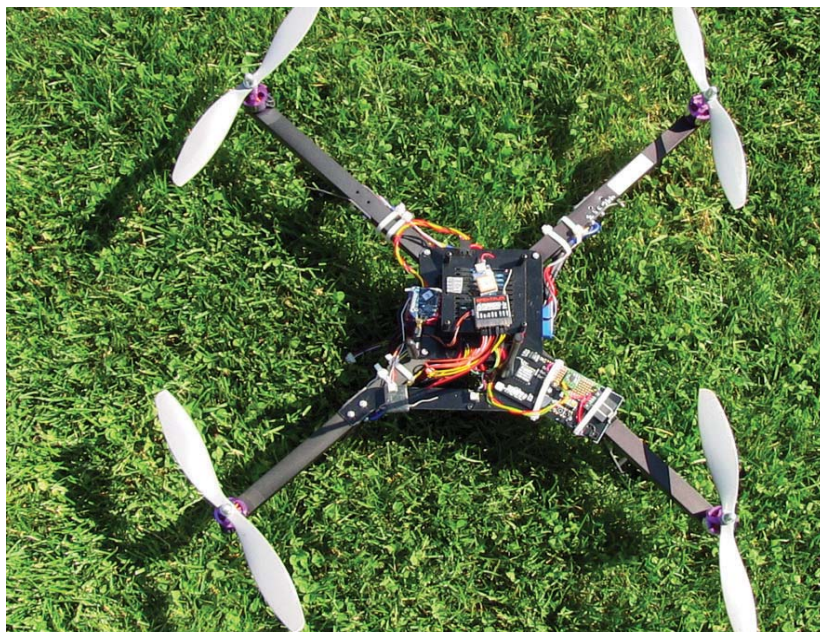
The commercial quadrotor (3D Robotics' ArduCopter) was modified to include a commercial receiver and Lincoln Laboratory–developed software.
