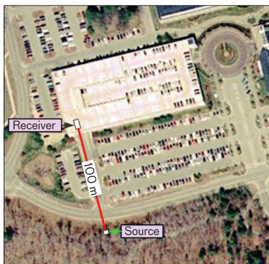
FIGURE 8. To provide truth data for the low-cost grating spectrometer, we colocated it with a high-fidelity FTIR. We released \text{SF}_6 at the source to ensure that both sensors viewed the same threat simulant. In the data from each instrument (right), the pink regions indicate when the gas was released. The concentration path length product (CL) in the middle plot is calculated from the FTIR data; the bottom plot shows the matched-filter output of the grating spectrometer. We saw a response for all six releases on the grating spectrometer, though one was below threshold. As expected, the noise was much higher in the grating system. For each release, we observed a positive spike corresponding to the threat detected, followed by a negative spike indicating that the threat had cleared. More sophisticated data processing and temperature stabilization should provide better performance. The plot at the top shows that the probability of false alarm declines as the detection threshold for triggering an alert is increased.
