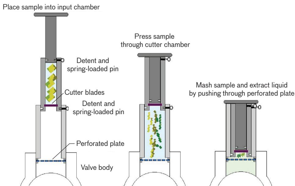
**FIGURE 14.** The tissue-grinding attachment initially chops the material into fine pieces. The mashing process compresses the solids and extracts the liquid, which proceeds into the sample chamber of the AMC.
