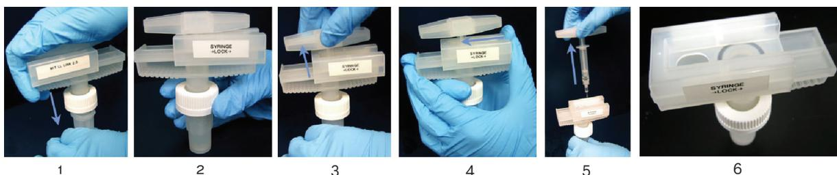
**FIGURE 19.** The post-sample-collection processing steps for the LiNK 2.0 are (1) insert the inner body into outer cylinder, filled with 2.0 mL water; (2) lock the cap; (3) load the syringe by pulling up on handle; (4) release the syringe by pressing the slider locking mechanism; (5) remove the syringe; and (6) push the slider to put LiNK 2.0 into the final closed position to seal the eluate into the unit for shipping/storage.
