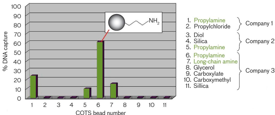
**FIGURE 5.** Screening of commercial-off-the-shelf (COTS) beads indicates the superior DNA adhesion to amine-based coatings (samples 1, 5, 6, and 7).
