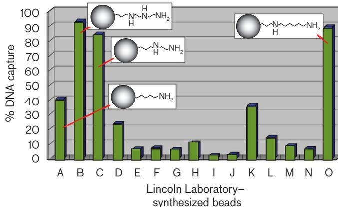
**FIGURE 6.** The Lincoln Laboratory–synthesized (LLS) bead coatings show similar results as the COTS beads with the best performance coming from amine-based functional groups (samples A, B, C, and O). Screening was done under identical conditions as the COTS beads.
