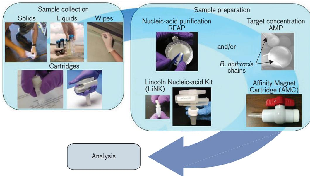
**FIGURE 1.** Two processing steps prior to analysis are addressed by our work. On the left are various sample-collection tools, including the Lincoln Nucleic-acid Kit (LiNK) version 1.0 and 2.0. On the right are the purification tools, which include LiNK family of cartridges, the Affinity Magnet Protocol (AMP) and the Recovery, Extraction, and Archiving Protocol (REAP).
