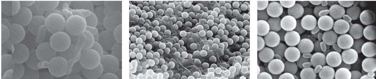
**FIGURE 7.** Scanning-electron-microscope images show COTS magnetic beads after being used to capture vegetative *Btk* cells (left), vegetative *Ba* cells (middle), and *Ba* spores (right). The bead target complexes were washed three times before imaging to remove non-adhered cells.
