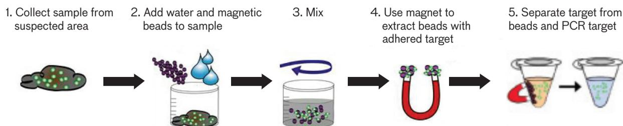
**FIGURE 3.** The AMP is used to isolate a target from a raw sample. The target is separated from the beads by using elution buffers, and the resulting material can be processed by polymerase chain reaction (PCR). This procedure has been implemented in a cartridge format.
