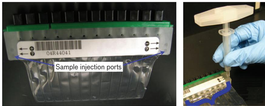
**FIGURE 20.** The vacuum-sealed RAZOR pouch, shown on the left, contains the thin flexible lower pouch section that is inserted into the RAZOR. Loading a sample into a RAZOR pouch, shown on the right, requires a controlled-aspiration syringe with a blunt cannula tip and a Lincoln Laboratory–designed custom handle.
