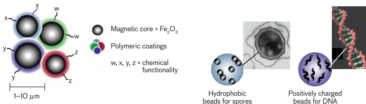
**FIGURE 4.** Magnetic beads with polymeric coatings are designed to attract and hold certain types of targets. Shown on the left is the structure of several beads, each designed with a specific chemical functionality. On the right are two conceptual images of bead coatings indicating the specificity of the design of the bead coatings to the surface properties of the targets.
