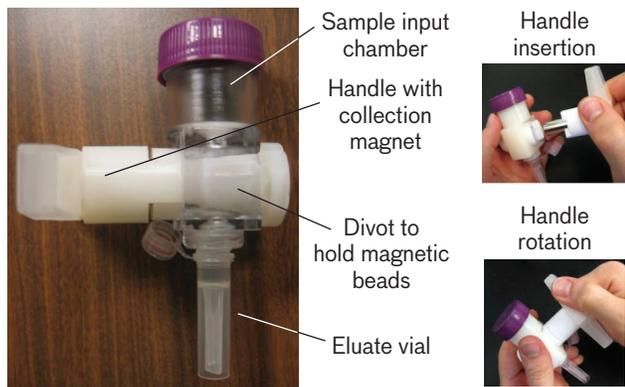
**FIGURE 11.** The one-valve custom AMC reduces the weight of multiple cartridges by utilizing a single handle that contains the reusable collection magnet.
