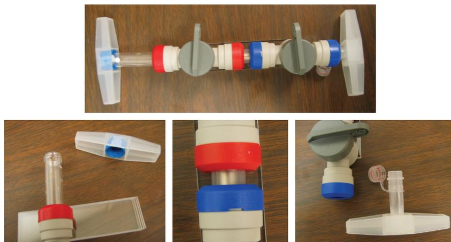
**FIGURE 9.** The two-valve AMC is based on COTS components. Shown at the top is the assembled cartridge. Below on the left is the polystyrene test-tube input chamber with the cap removed. In the center is the polypropylene test-tube processing chamber with the collection magnet (a radially magnetized chrome-plated neodymium-boron rare-earth cylinder) inside the chamber. On the right is the eluate chamber, a 1.5 mL cryogenic-compatible storage vial, with the attached cap and handle.
