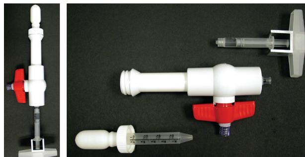
**FIGURE 12.** The assembled (left) and disassembled (right) AMC shows the dropper attachment to the input chamber, the syringe, and the one-way valve attachment to the output end. The cartridge body has an extension on the input chamber to accommodate the dropper, and the syringe has an attached handle for eluate removal (top right).
