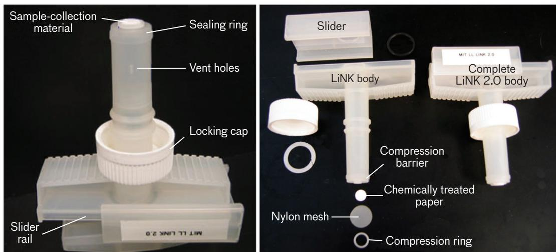
**FIGURE 18.** The LiNK 2.0 prototype assembly has all the components necessary for processing samples. On the left is the inner body. On the right is an exploded view of the inner body with components and a completely assembled unit.
