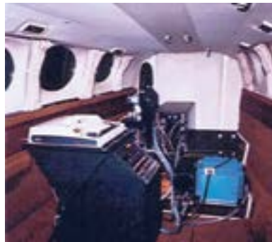
The Lincoln Laboratory TCAS experimental unit flew in a Cessna 421.
