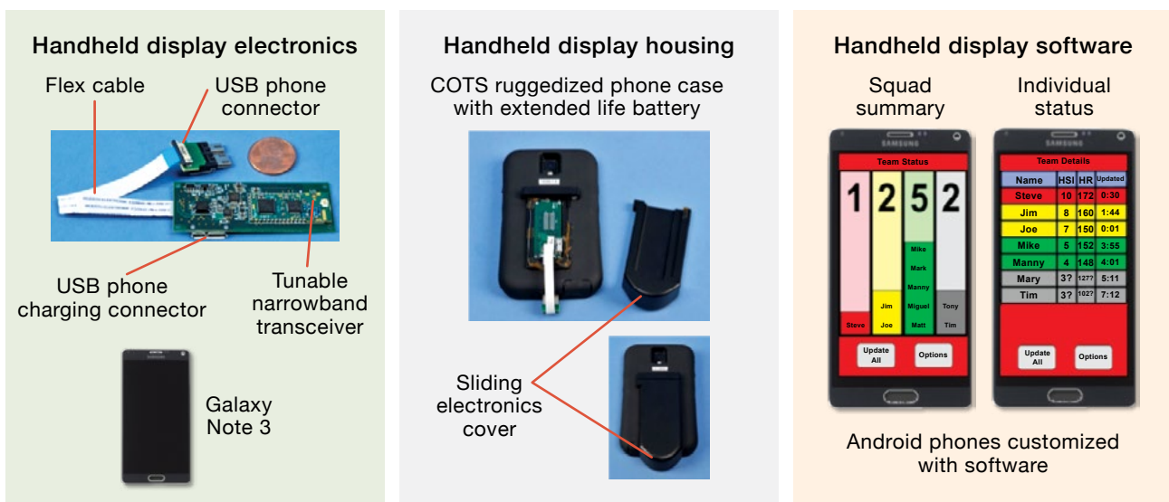
FIGURE 5. The prototype end-user device for the Open Body Area Network Physiological Status Monitor uses commercial off-the-shelf (COTS) components that were adapted for use with custom software and radio hardware.
