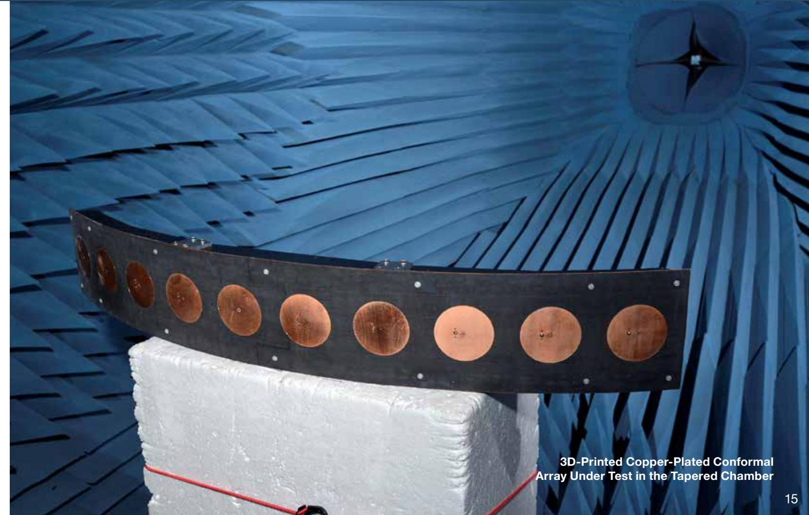
3D-Printed Copper-Plated Conformal Array Under Test in the Tapered Chamber
