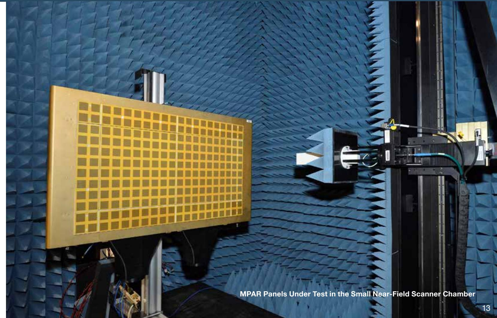
MPAR Panels Under Test in the Small Near-Field Scanner Chamber
