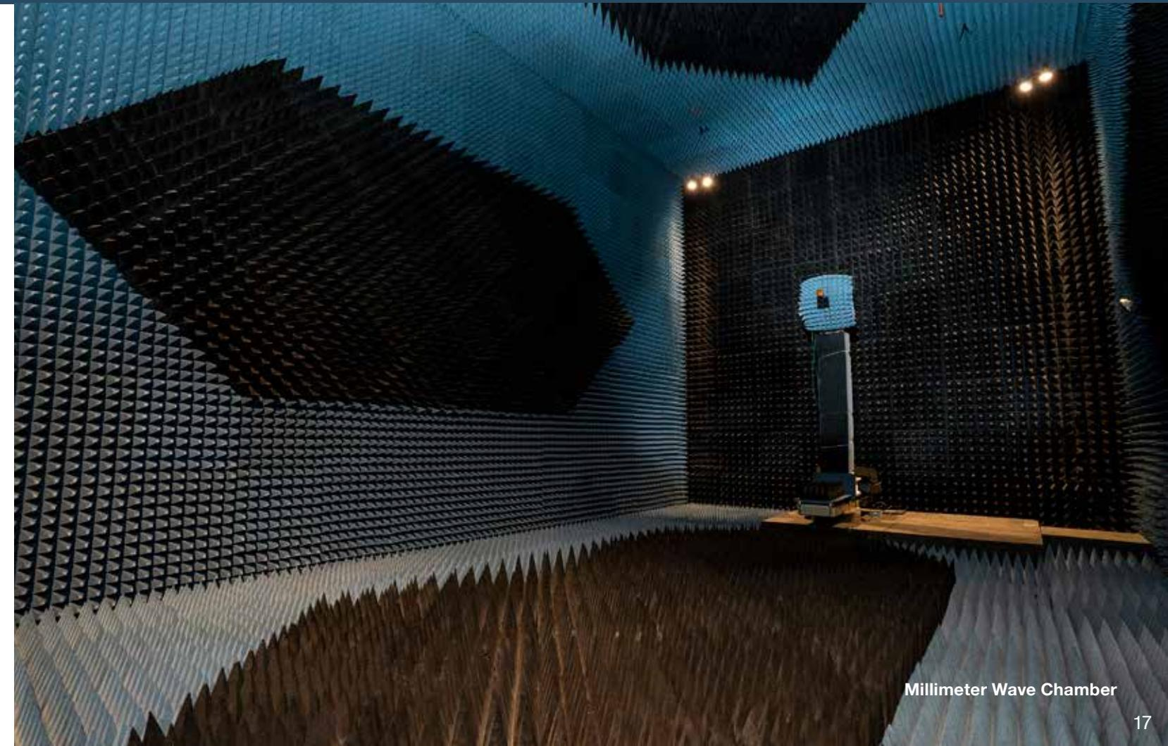
Millimeter Wave Chamber
