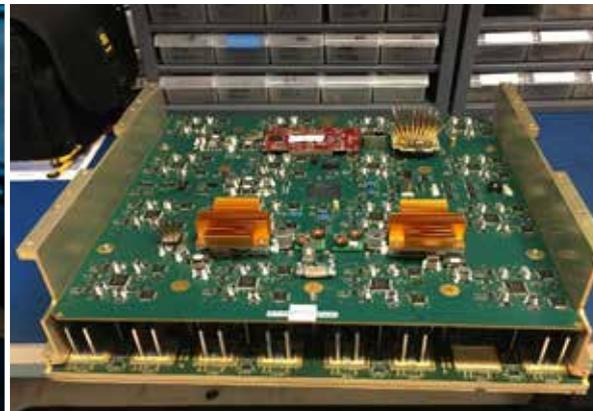
Active Electronically Scanned Antenna Panel
