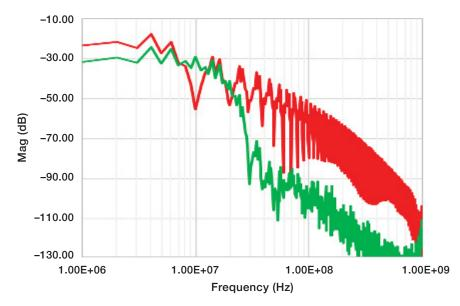
The plot shows that the SEDL circuit (green) uses less spectral energy (i.e., has lower decibel, dB, magnitude) than does the traditional logic circuit (red) at a range of frequencies. The lower spectrum usage means less EMI is generated by the circuit.
