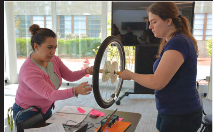
Esmeralda Hernandez (left) and Liz Raine spin a wheel above a small self-built radar system to determine the wheel's speed based on the Doppler effect.
