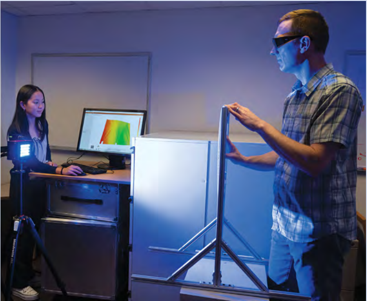
AFCEA intern Jessica Chan used a digital image correlation system to measure deformations in the membrane stretched by Mark Silver, Chan’s mentor. The two cameras turn pictures of the membrane into data representing the membrane’s movement.
