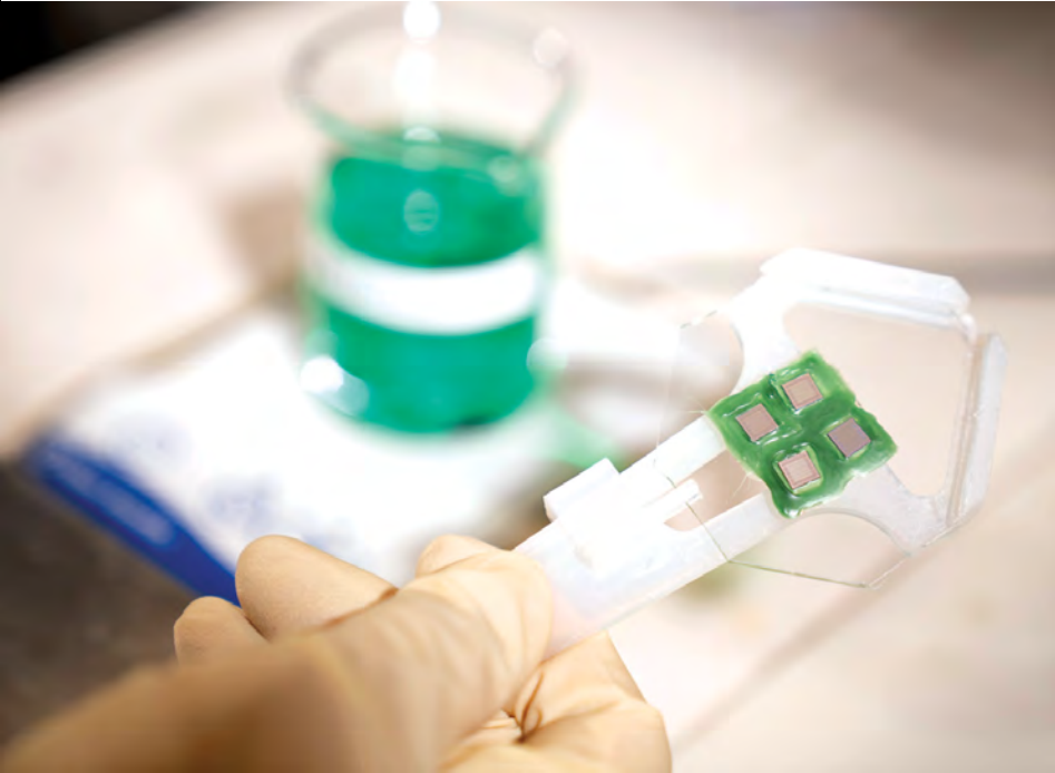
Above, a close-up view of the custom ROIC is shown here. At left, four custom ROICs have been mounted so that they can be placed on metal plating. The GmAPDs are layered onto this circuit, and they work together to capture and record the photon signals.
