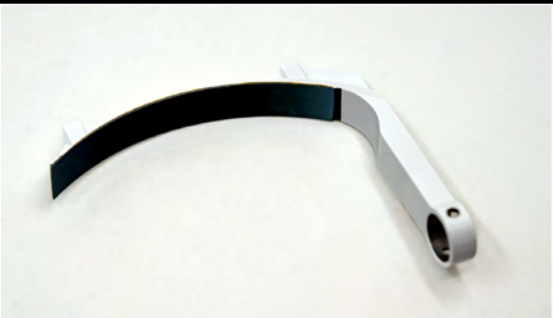
The occulter, shown here, is fabricated from aluminum following the same process used on the baffle.
