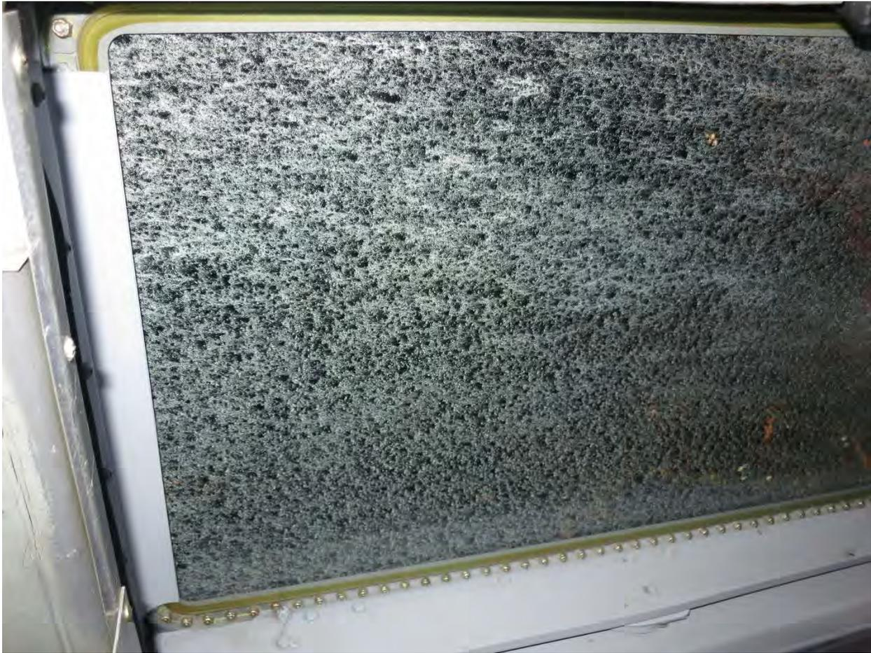
*Figure 19. Image showing the accumulation of supercooled raindrops frozen onto the side window of the Convair-580.*
