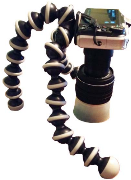
Figure A-5. Camera apparatus for imaging frozen particles.
