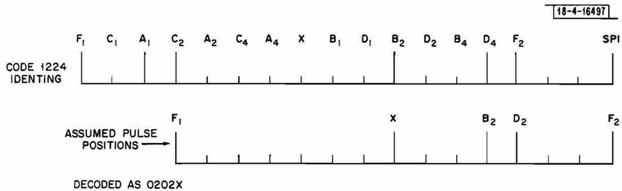
Fig. 10. Generation of a  $C_2$  - SPI Phantom.
