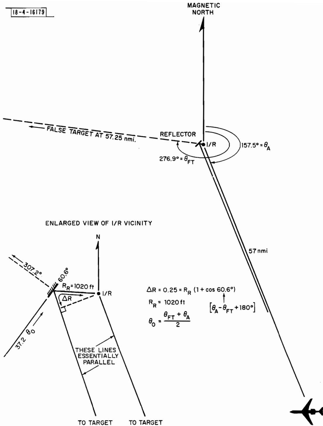
Fig. 11. Simplified geometry  $R_A \gg R_R$ .
