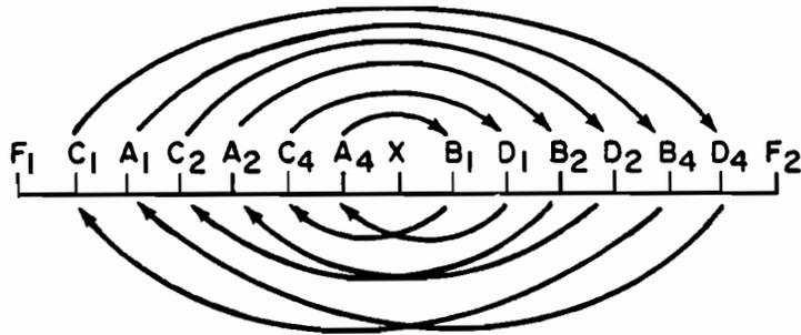
Fig. 36 Relationship between anomalous and legitimate reply pulses.
