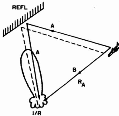
Fig. 24. Sidelobe reply processing.
