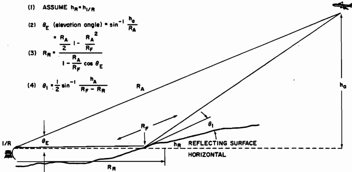
$$h_o = h_{\text{reported}} + h_{\text{earth curvature}} - h_{I/R}$$
