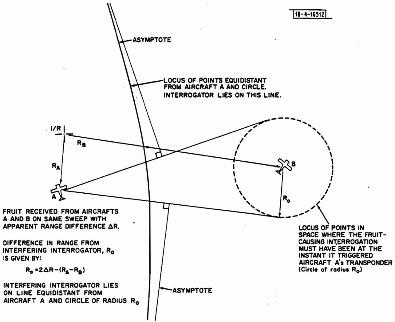
Fig. 30. Direction-finding from multiple fruit on a sweep.
