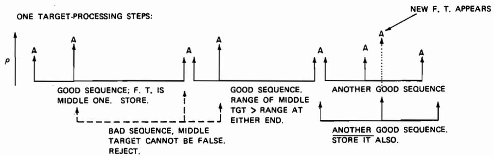
Fig. 19. Discrete-code false target processing.
