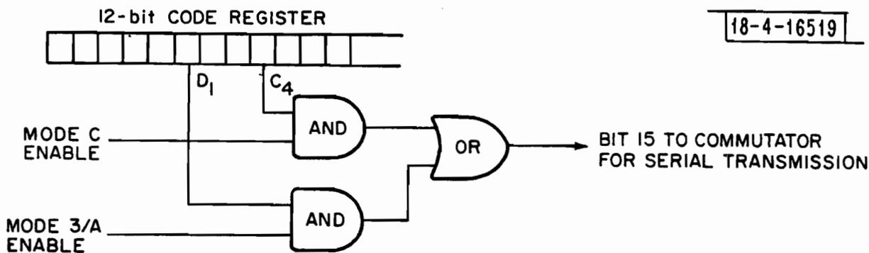
Fig. 37 ARTS III Reply Code Readout Circuitry
