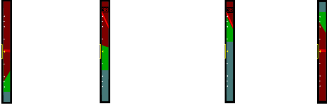
Figure 1. Examples of TCAS vertical speed displays for some common RAs. Far left: “Descend, Descend.” Center left: “Adjust Vertical Speed, Adjust” (0 fpm). Center right: “Adjust Vertical Speed, Adjust” (2000 fpm). Far right: “Climb, Climb.” The aircraft’s current vertical speed is indicated by the bright red needle on the instrument. [6]
