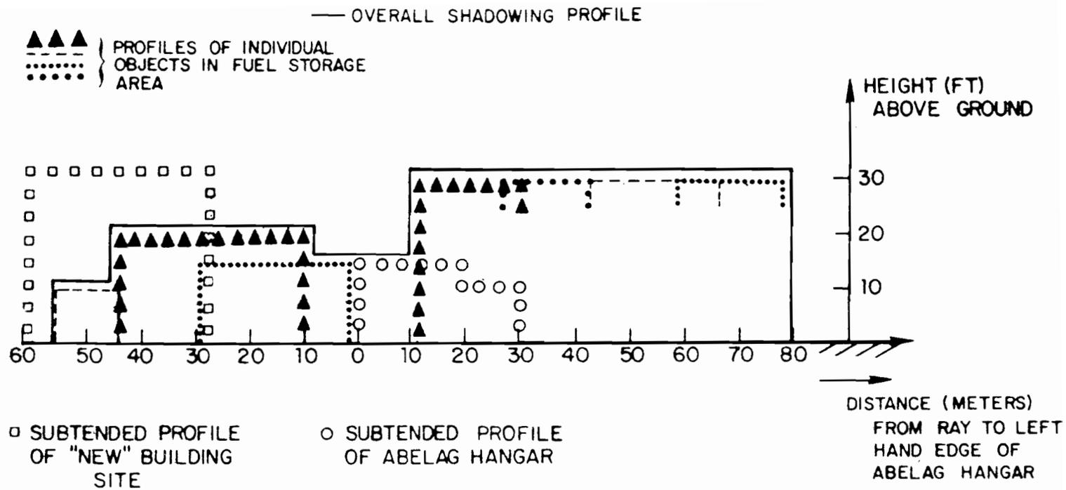
Fig. 6-53. Inferred shadowing profile of fuel storage area.
