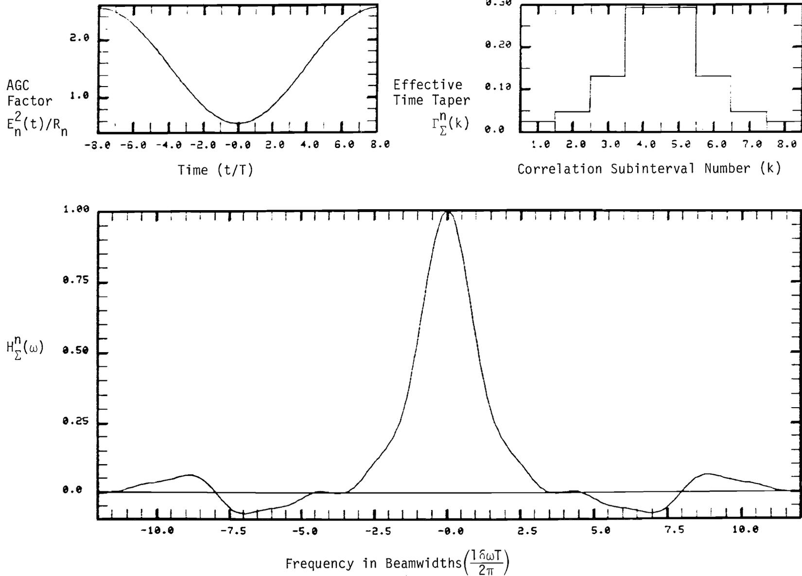
Fig. 6-13. Sum filter frequency response for scalloping frequency of  $\frac{2\pi}{16T}$  (420 Hz) and midscan phase of  $180^\circ$ .
