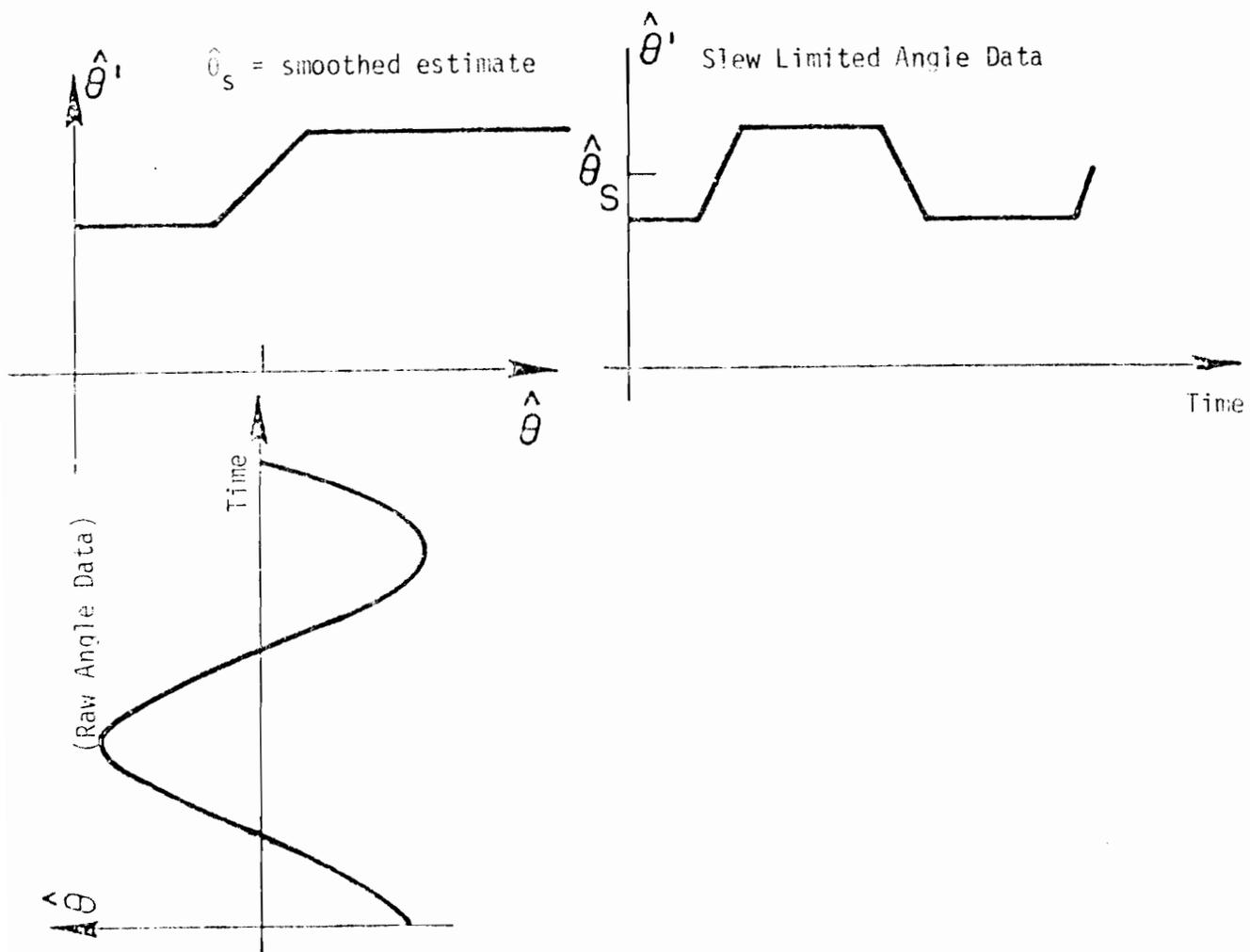
Fig. 5-3. Input-output time waveforms with TRSB Phase II receiver slew limiter.
