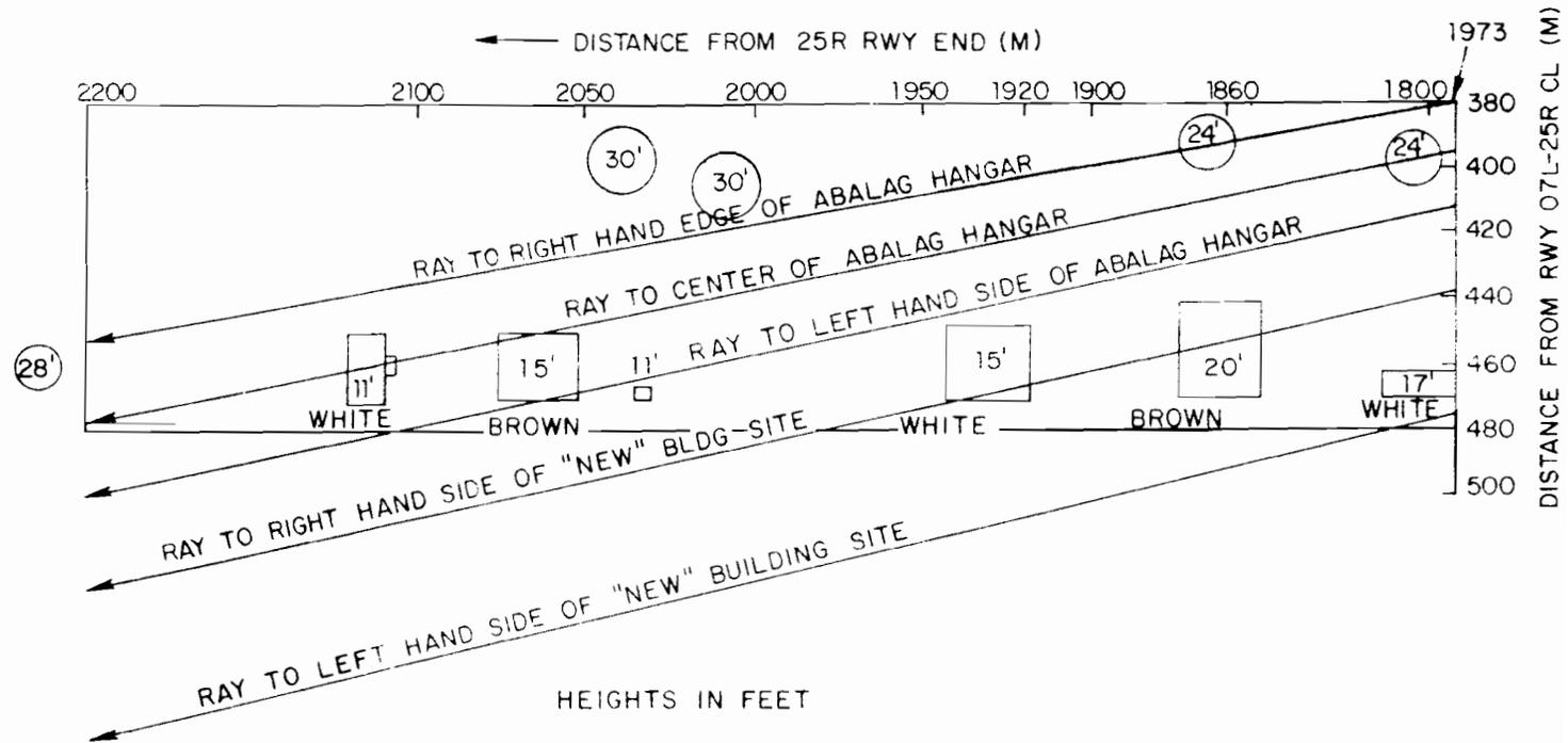
Fig. 6-51. Inferred fuel storage area structure locations and heights.
