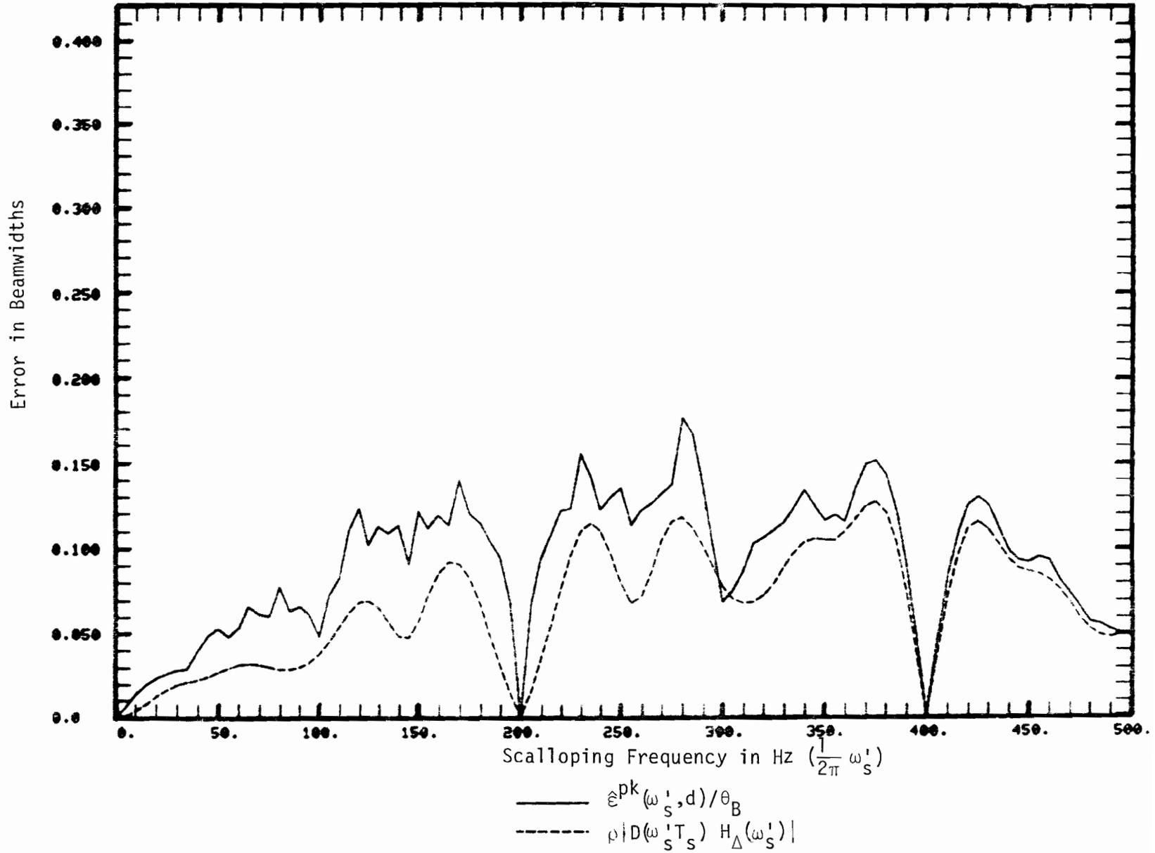
Fig. 6-25. Motion averaged errors for scan sequence #237 (++++---+---+).
