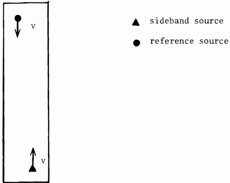
Both sources simultaneously move at velocity  $v$  towards opposite end of the array.
