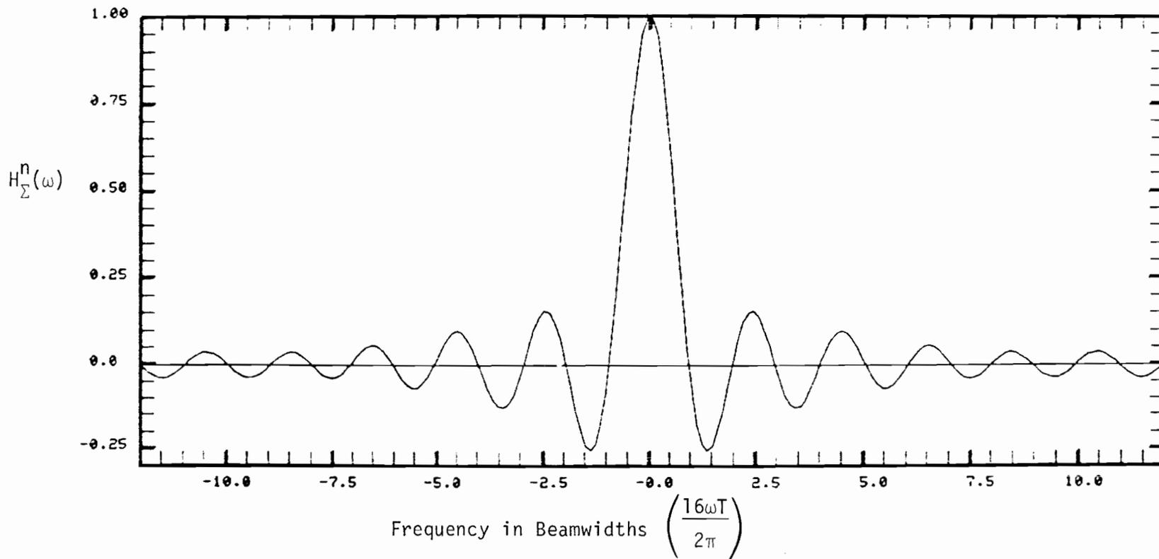
Fig. 6-9. Sum filter frequency response for scalloping frequency of  $\frac{2\pi}{16T}$  (420 Hz) and midscan phase of  $0^\circ$ .
