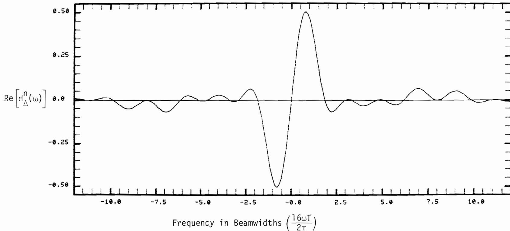
Fig. 6-12(a). Real part of difference filter frequency response for scalloping frequency of  $\frac{2\pi}{16T}$  (420 Hz) and midscan phase of  $90^\circ$ .
