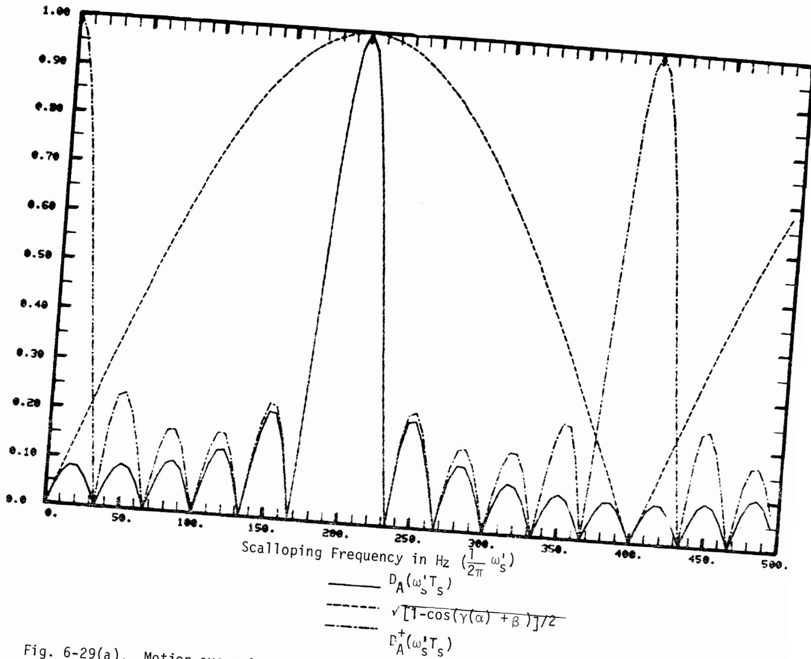
Fig. 6-29(a). Motion averaging factor for alternating scan sequence  $d_A(n)$  (+--+--+--+--+)
