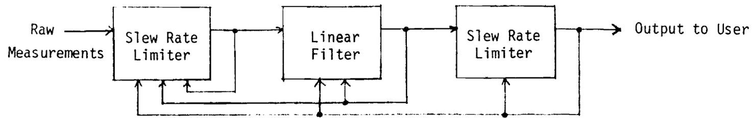
Fig. 5-1. Data editing structure employing slew rate limiters.
