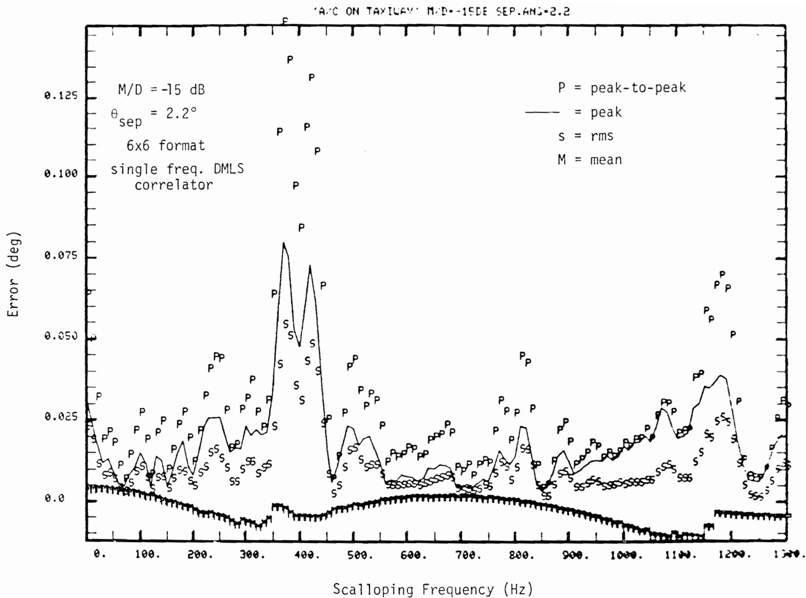
Fig. 6-33. DMLS dynamic error for out-of-beam azimuth multipath.
