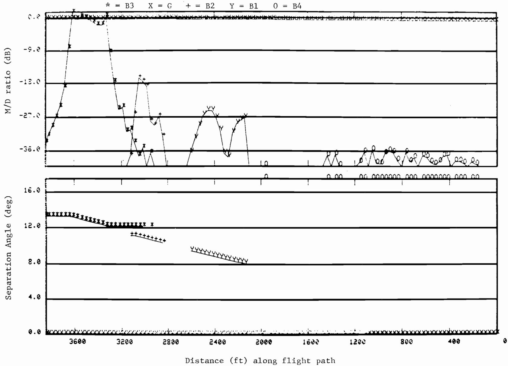
Fig. 6-44. Azimuth multipath characteristics for scenario of Fig. 6-43.
