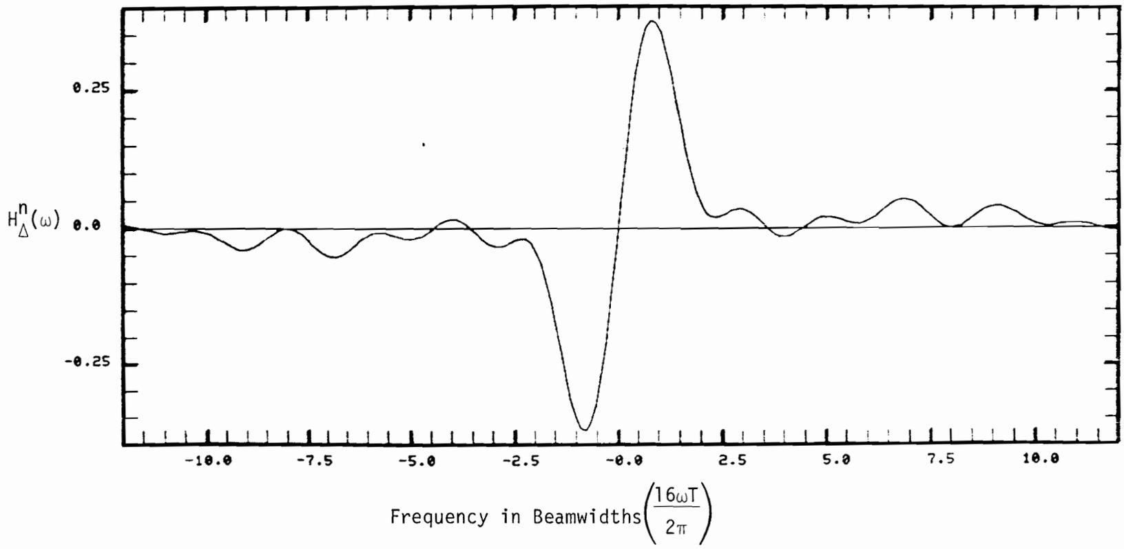
Fig. 6-8. Difference filter frequency response for scalloping frequency of  $\frac{1}{2} \frac{2\pi}{16T}$  (210 Hz) and midscan phase of  $180^\circ$ .
