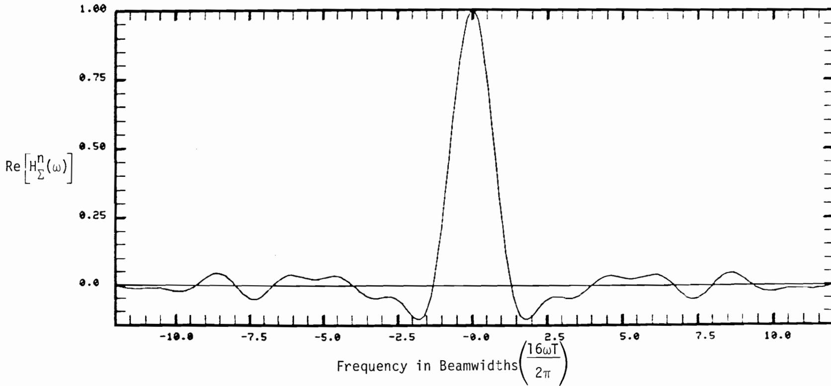
Fig. 6-11(a). Real part of sum filter frequency response for scalloping frequency of  $\frac{2\pi}{16T}$  (420 Hz) and midscan phase of  $90^\circ$ .
