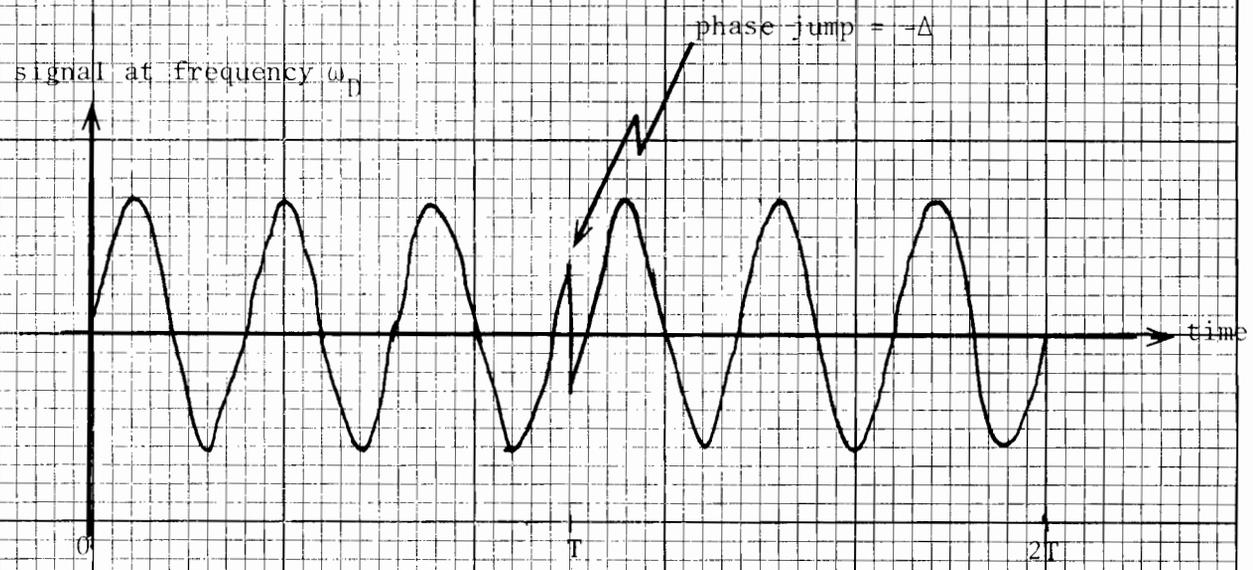
$\phi =$  rf phase between direct and multipath at time  $t=T$
