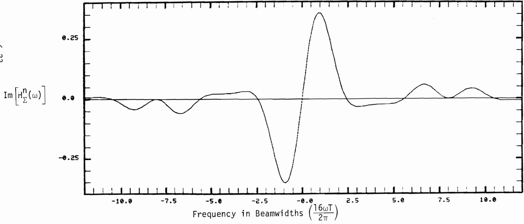
Fig. 6-11(b). Imaginary part of sum filter frequency response for scalloping frequency of  $\frac{2\pi}{16T}$  (420 Hz) and midscan phase of  $90^\circ$ .
