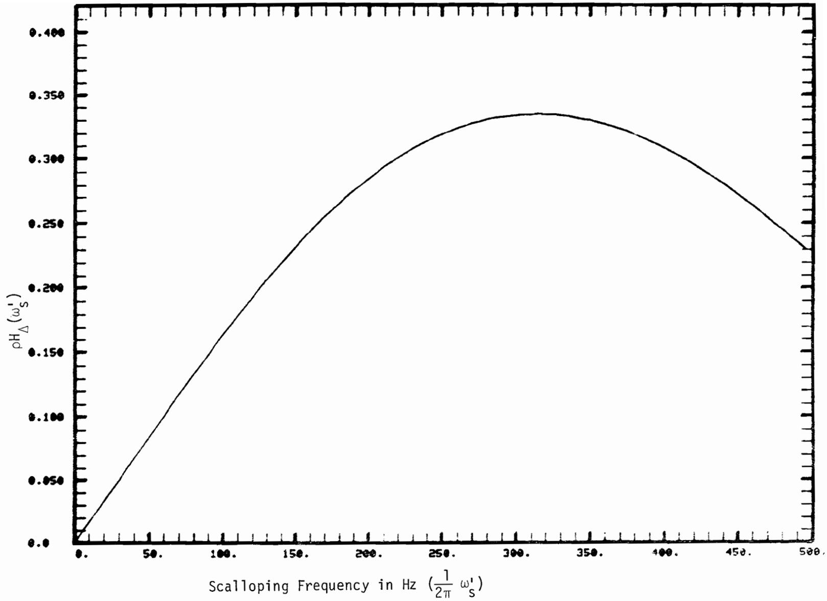
Fig. 6-21. First-order static error characteristic,  $\rho_{H\Delta}(\omega'_S)$ .
