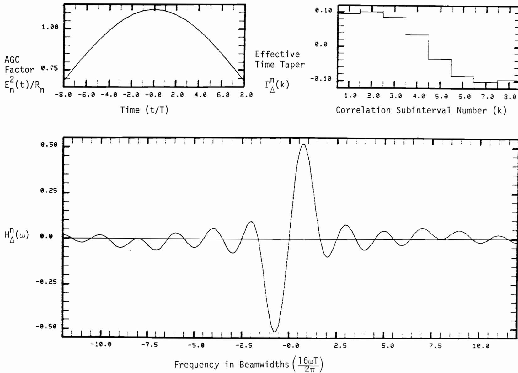
Fig. 6-4. Difference filter frequency response for scalloping frequency of  $\frac{1}{2} \frac{2\pi}{16T}$  (210 Hz) and midscan phase of  $0^\circ$ .
