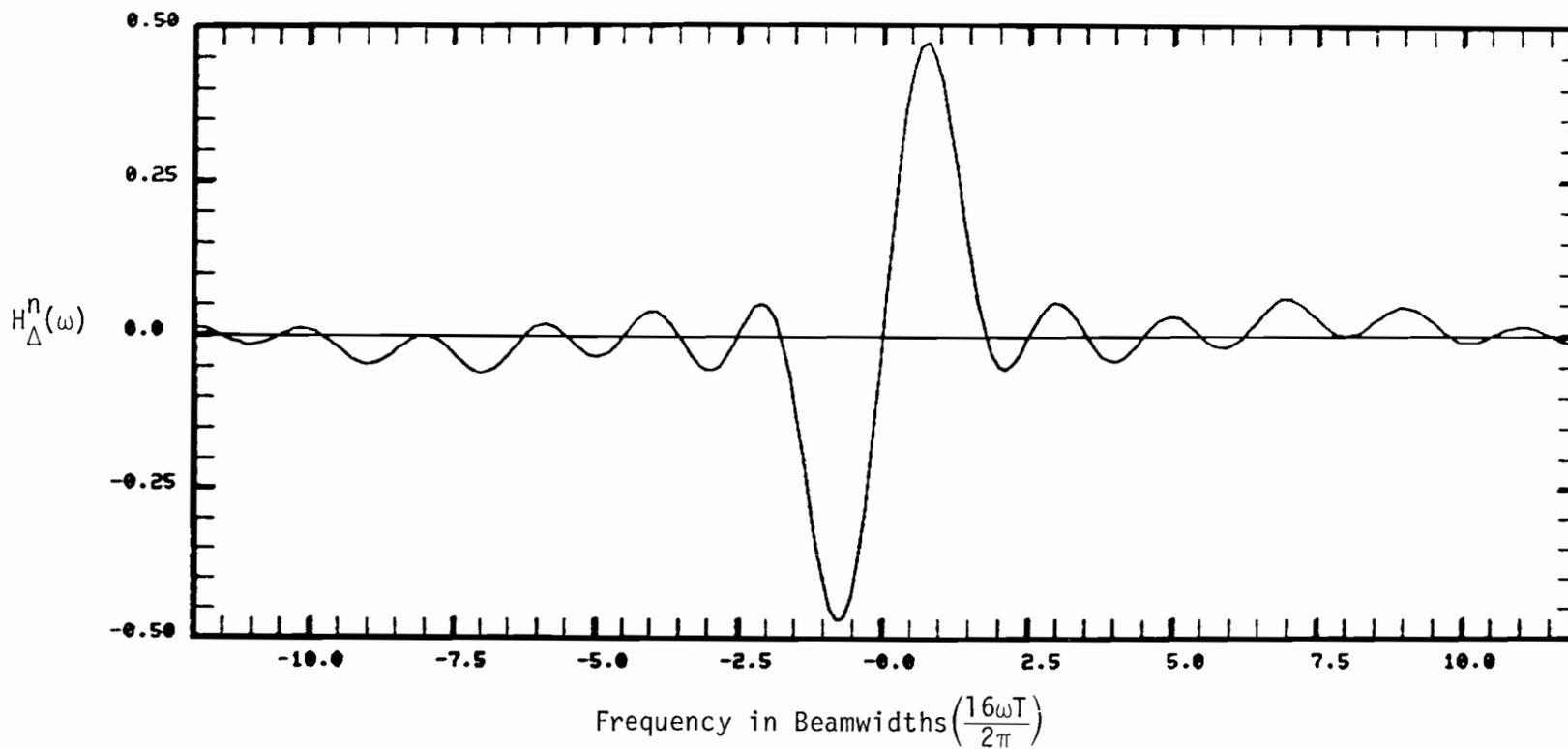
Fig. 6-2. Difference filter frequency response for zero scalloping frequency (uniform AGC factors).
