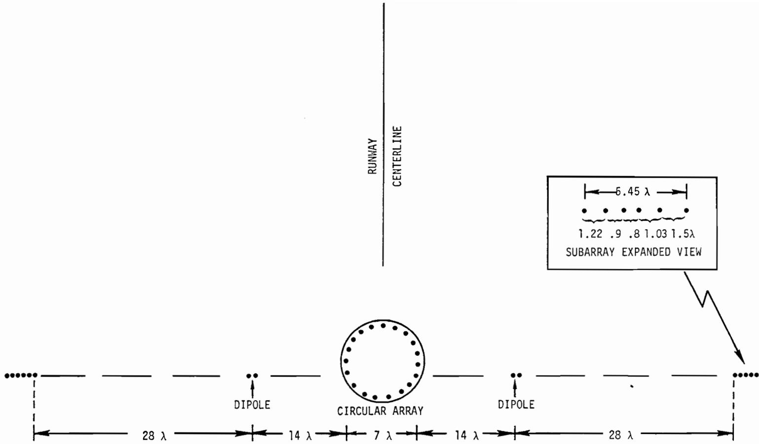
Fig. B-1. DLS azimuth antenna configuration.
