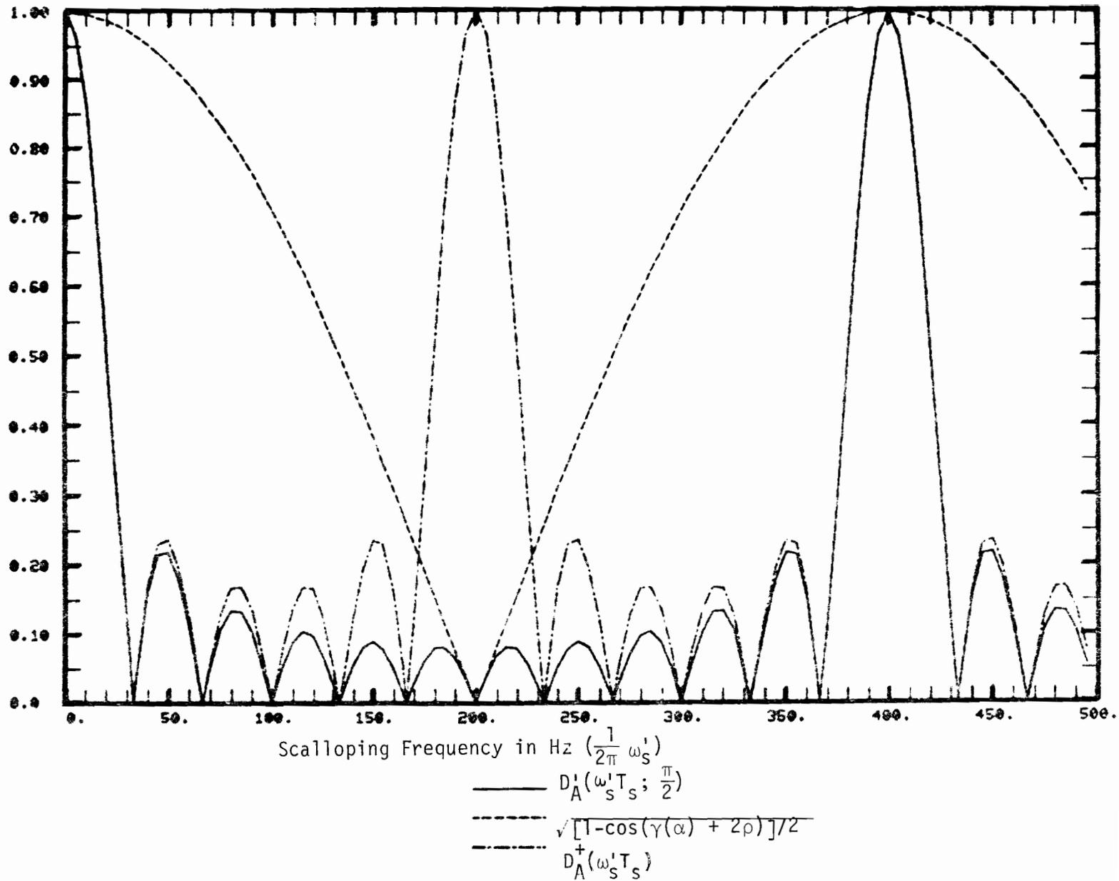
Fig. 6-29(b). Motion averaging factor for alternating scan sequence  $d_A(n)$  (+--+--+--+--+--) with multipath time delay of 6  $\mu$ sec.
