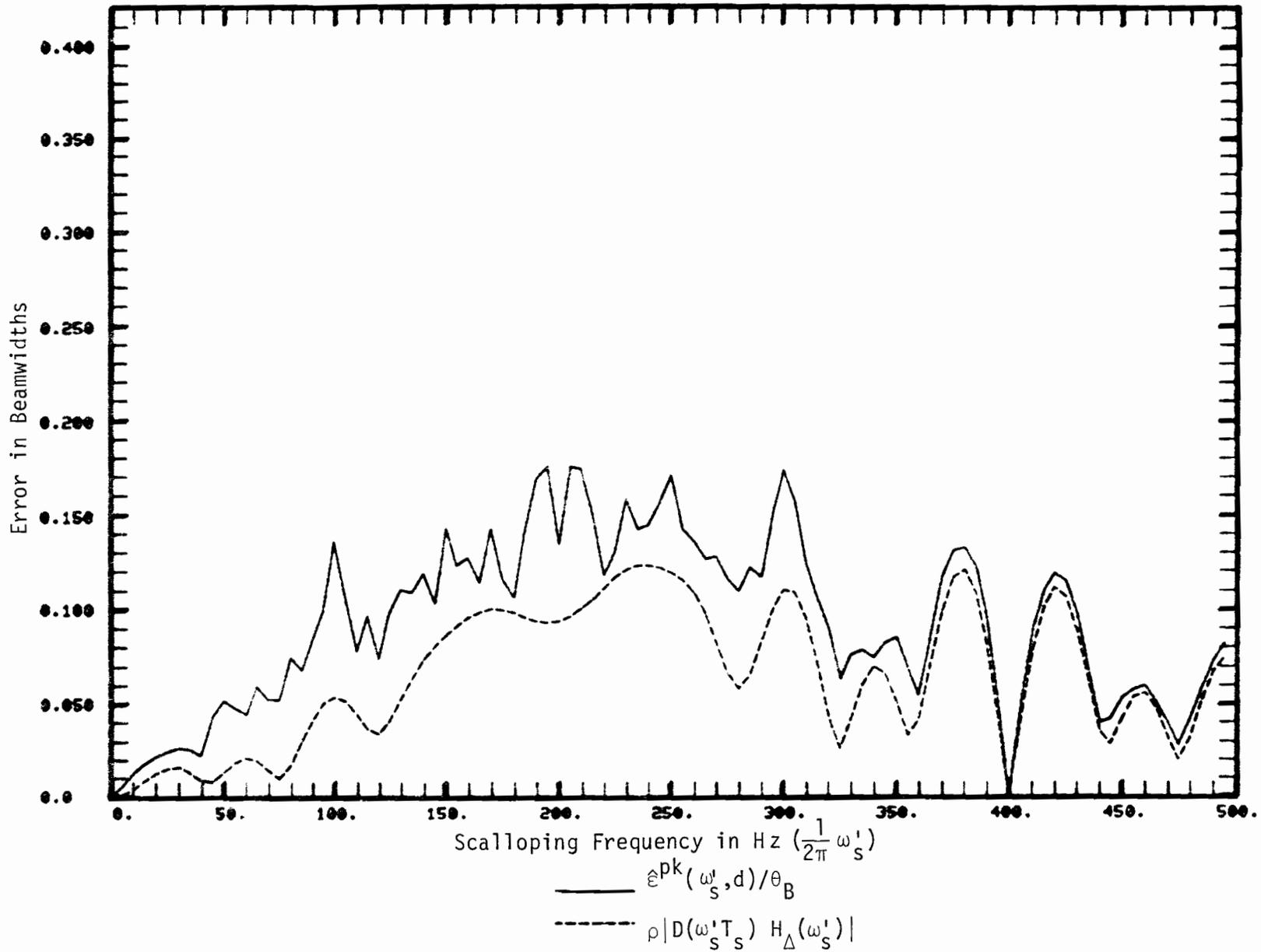
Fig. 6-26. Motion averaged errors for scan sequence #347 (++++-+----).
