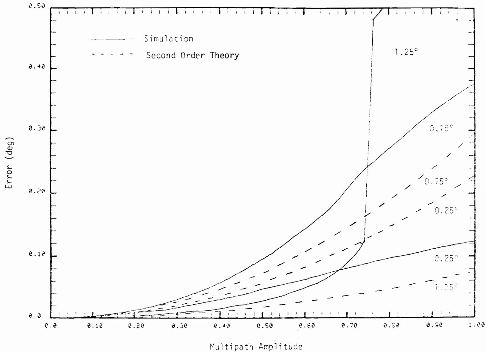
Fig. 5-6. Slew bias error vs. multipath amplitude for various separation angles.
