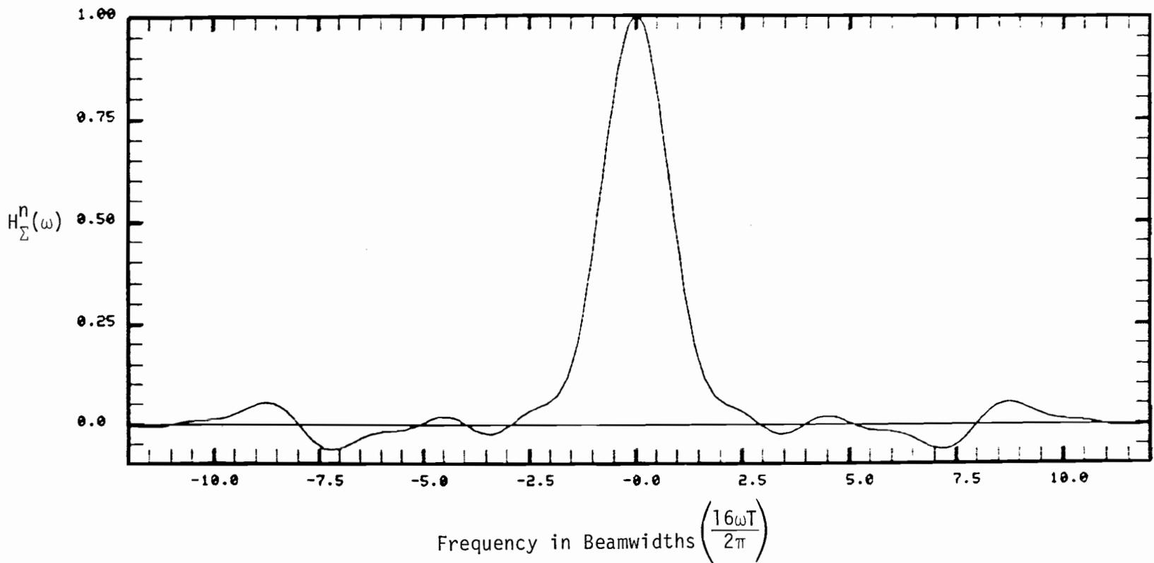
Fig. 6-7. Sum filter frequency response for scalloping frequency of  $\frac{1}{2} \frac{2\pi}{16T}$  (210 Hz) and midscan phase of  $180^\circ$ .
