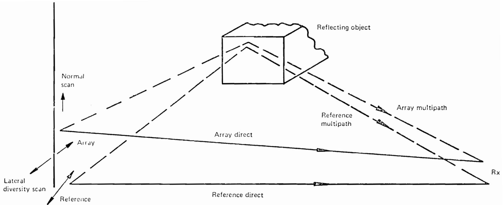
Fig. 6-38. Lateral diversity elevation with reflective object (from [7]).
