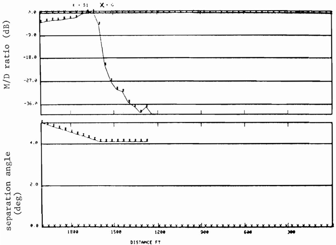
Fig. 6-63. Azimuth multipath characteristics for array scalloping scenario.
