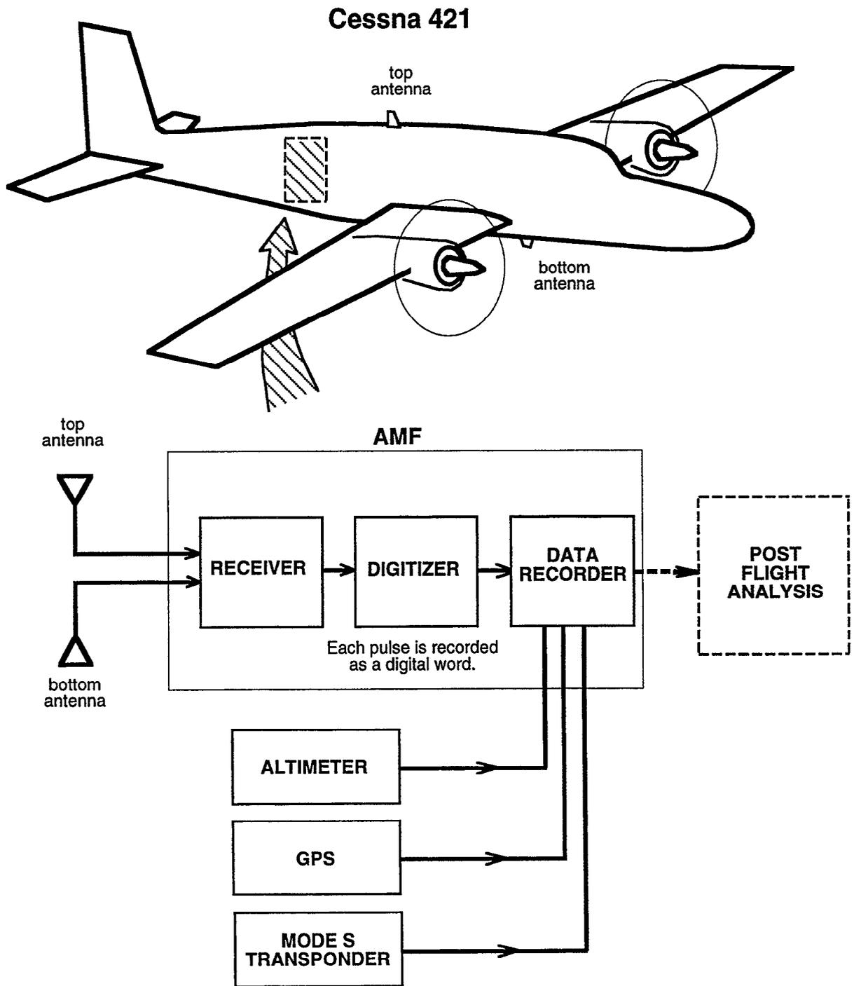
*Figure 1. The Airborne Measurement Facility.*
