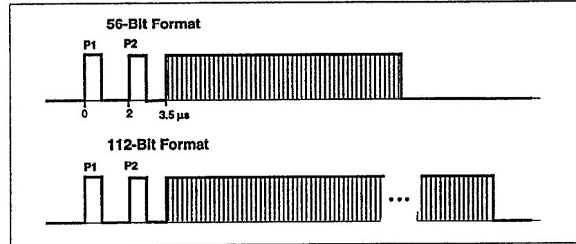
Figure 2. Transmissions in the 1030 MHz band.
