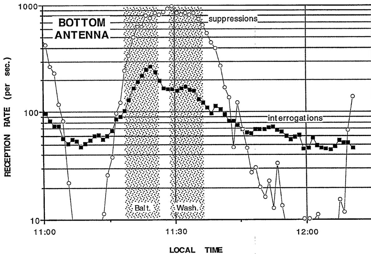
Figure 11. Total interrogations and suppressions received by the AMF (Washington).
