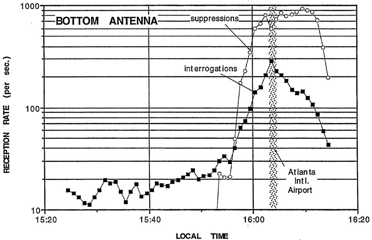
Figure 15. Total interrogations and suppressions received by the AMF (Atlanta).
