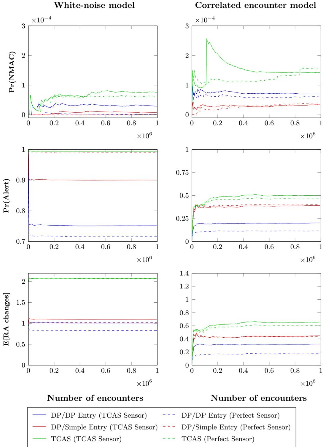
Figure 28. Convergence curves for DP and TCAS with and without sensor noise.
