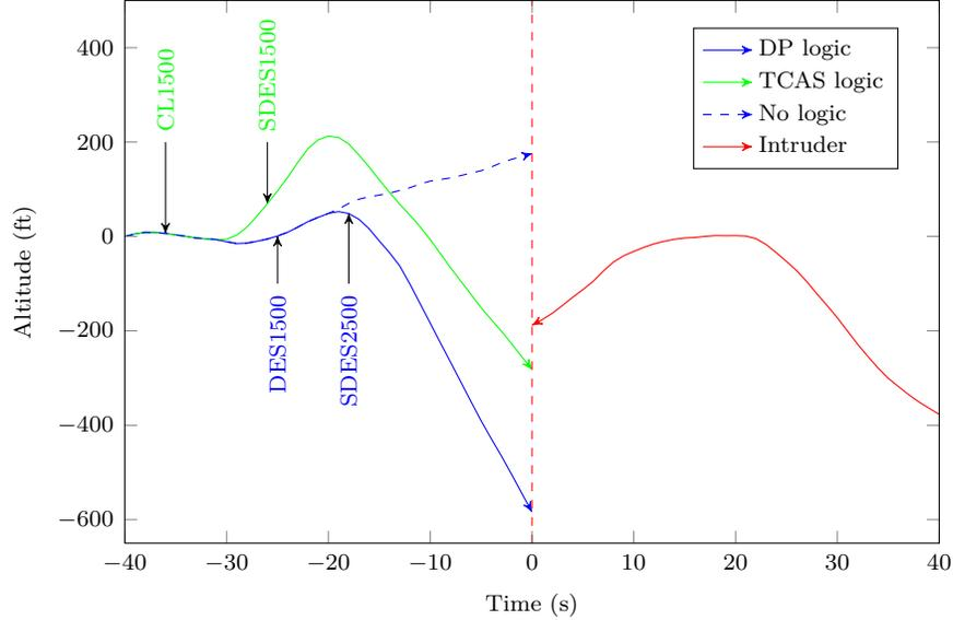
Figure 5. Example encounter comparing the performance of the DP logic against the current TCAS logic. The own aircraft approaches from the left, and the intruder approaches from the right.
