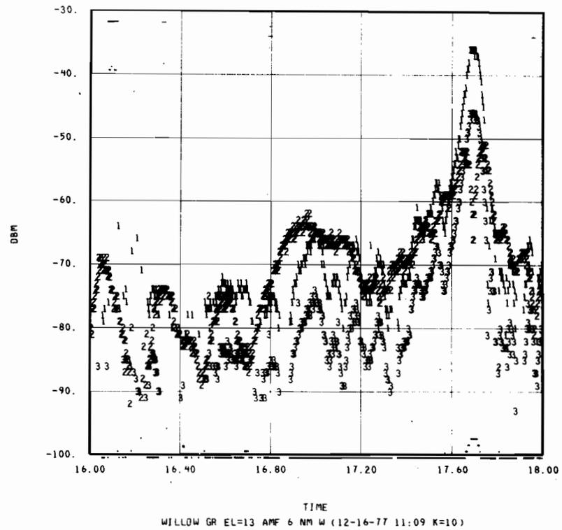
Fig. 3-1c. Antenna Pattern, Detail - Willow Grove, 14.00-18.00 Secs.
