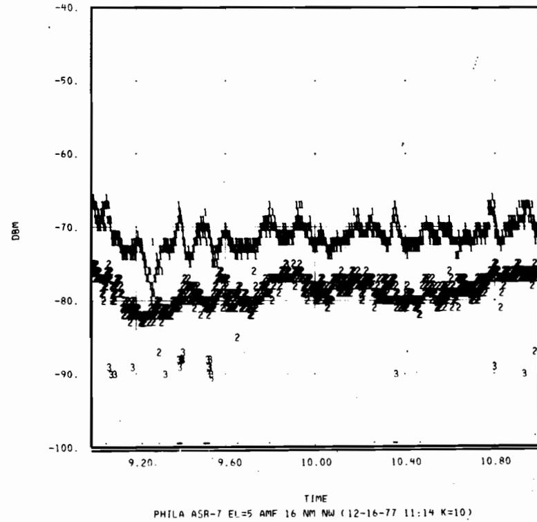
Fig. 3-2d. Antenna Pattern, Detail - Philadelphia (ASR-7), 7.20-10.80 Secs.
