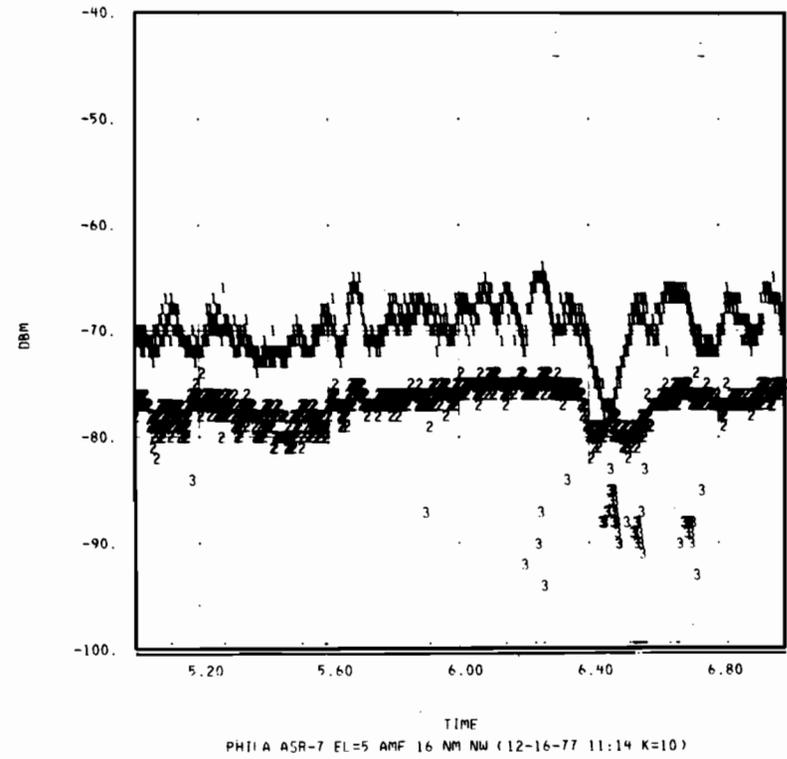
Fig. 3-2c. Antenna Pattern, Detail - Philadelphia (ASR-7), 3.20-6.80 Secs.
