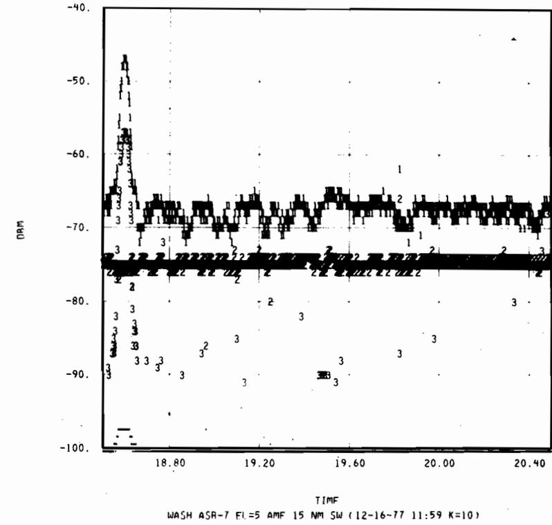
Fig. 3-3e. Antenna Pattern, Detail - Washington (ASR-7), 16.80-20.40 Secs.
