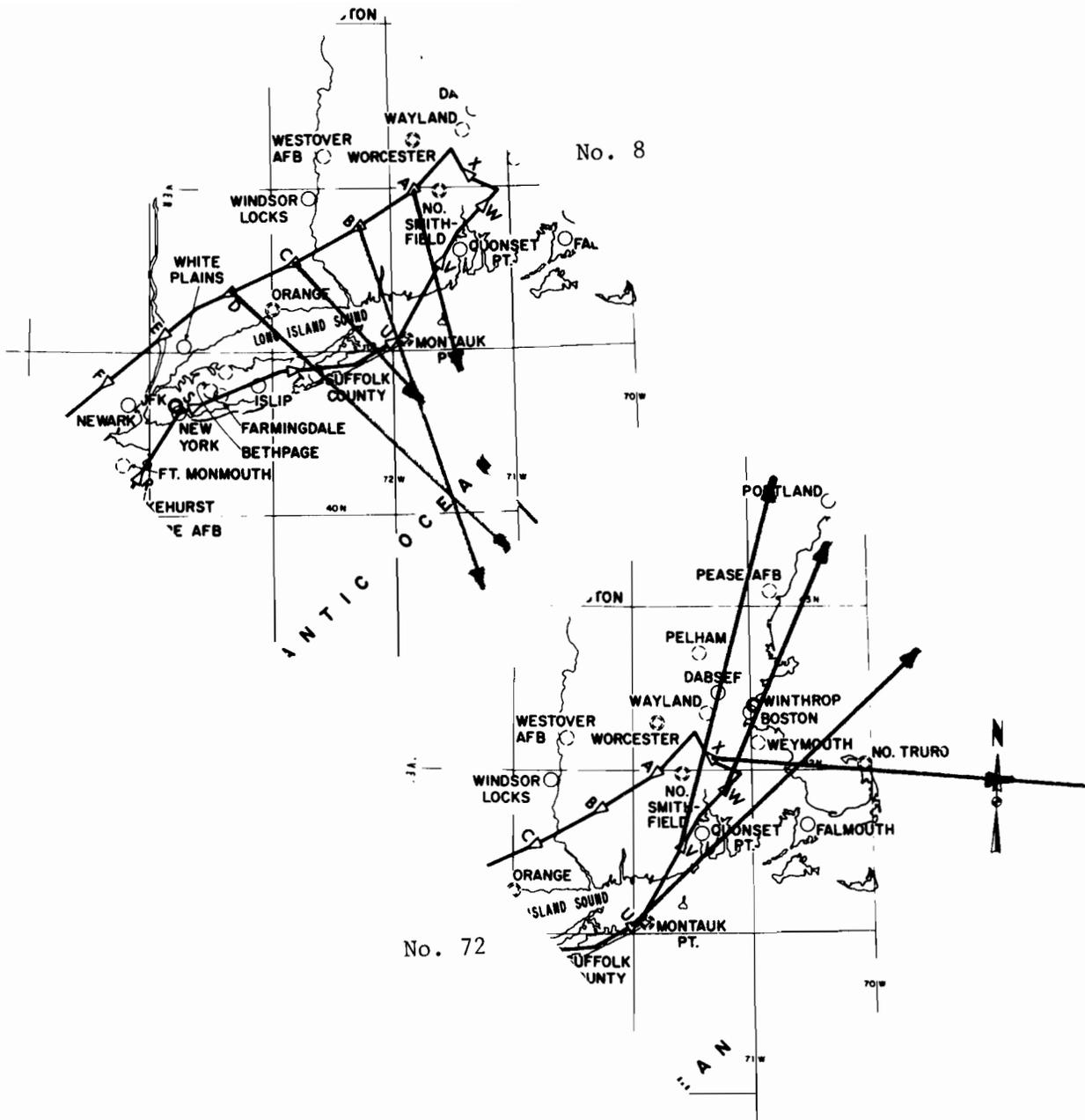
Fig. 2-1f. Angle-of-Arrival Rays for Unidentified Interrogators 3 and 72.
