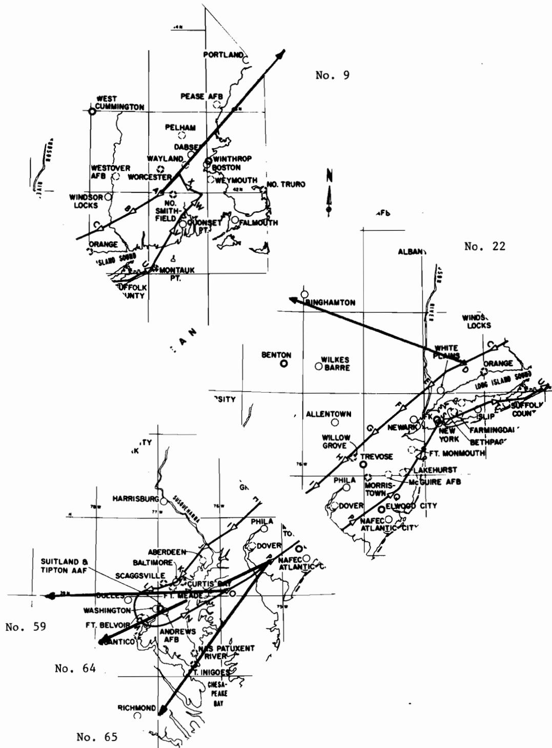
Fig. 2-1a. Angle-of-Arrival Rays for Unidentified Interrogators 9, 22, 59, 64 and 65.
