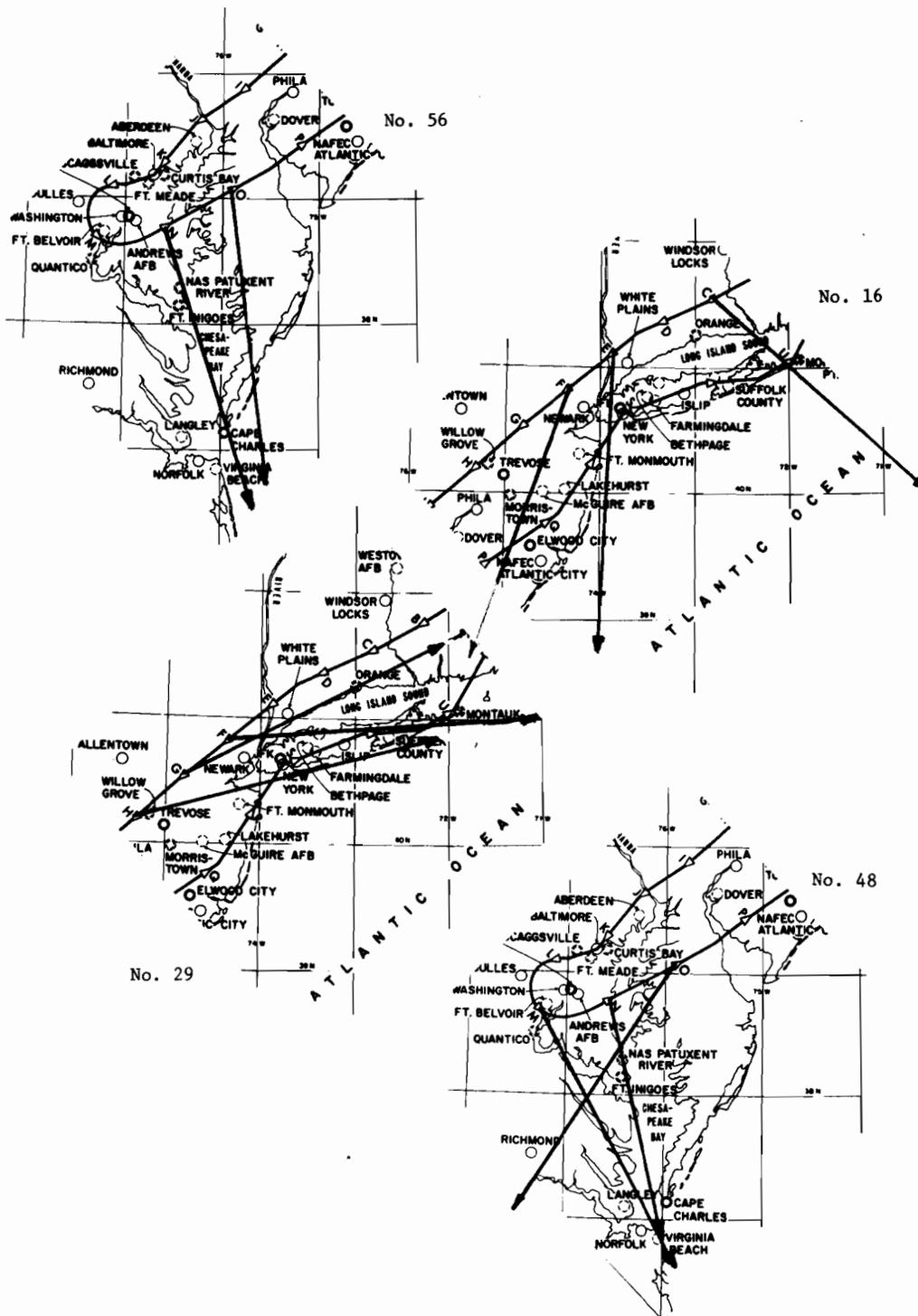
Fig. 2-1c. Angle-of-Arrival Rays for Unidentified Interrogators 16, 29, 48 and 56.
