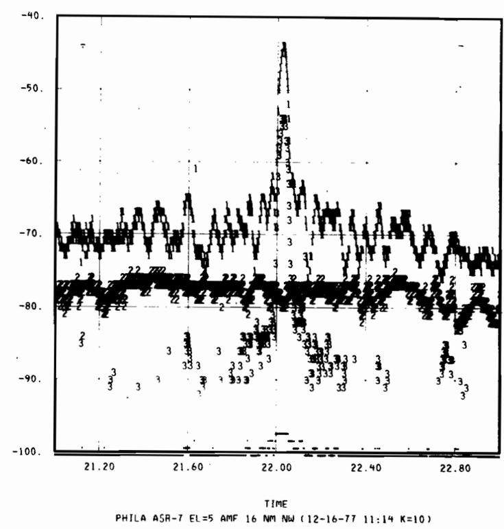
Fig. 3-2g. Antenna Pattern, Detail - Philadelphia (ASR-7), 19.20-22.80 Secs.
