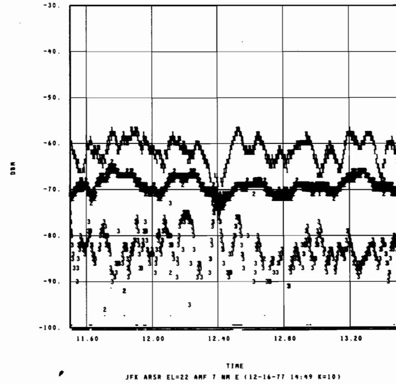
Fig. 3-4d. Antenna Pattern, Detail - JFK-NY (ARSR), 9.60-13.20 Secs.
