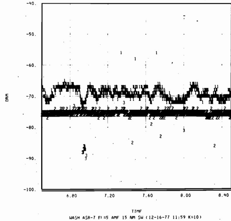
Fig. 3-3b. Antenna Pattern, Detail - Washington (ASR-7), 4.80-8.40 Secs.
