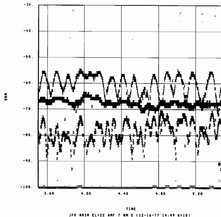
Fig. 3-4b. Antenna Pattern, Detail - JFK-NY (ARSR), 1.60-5.20 Secs.
