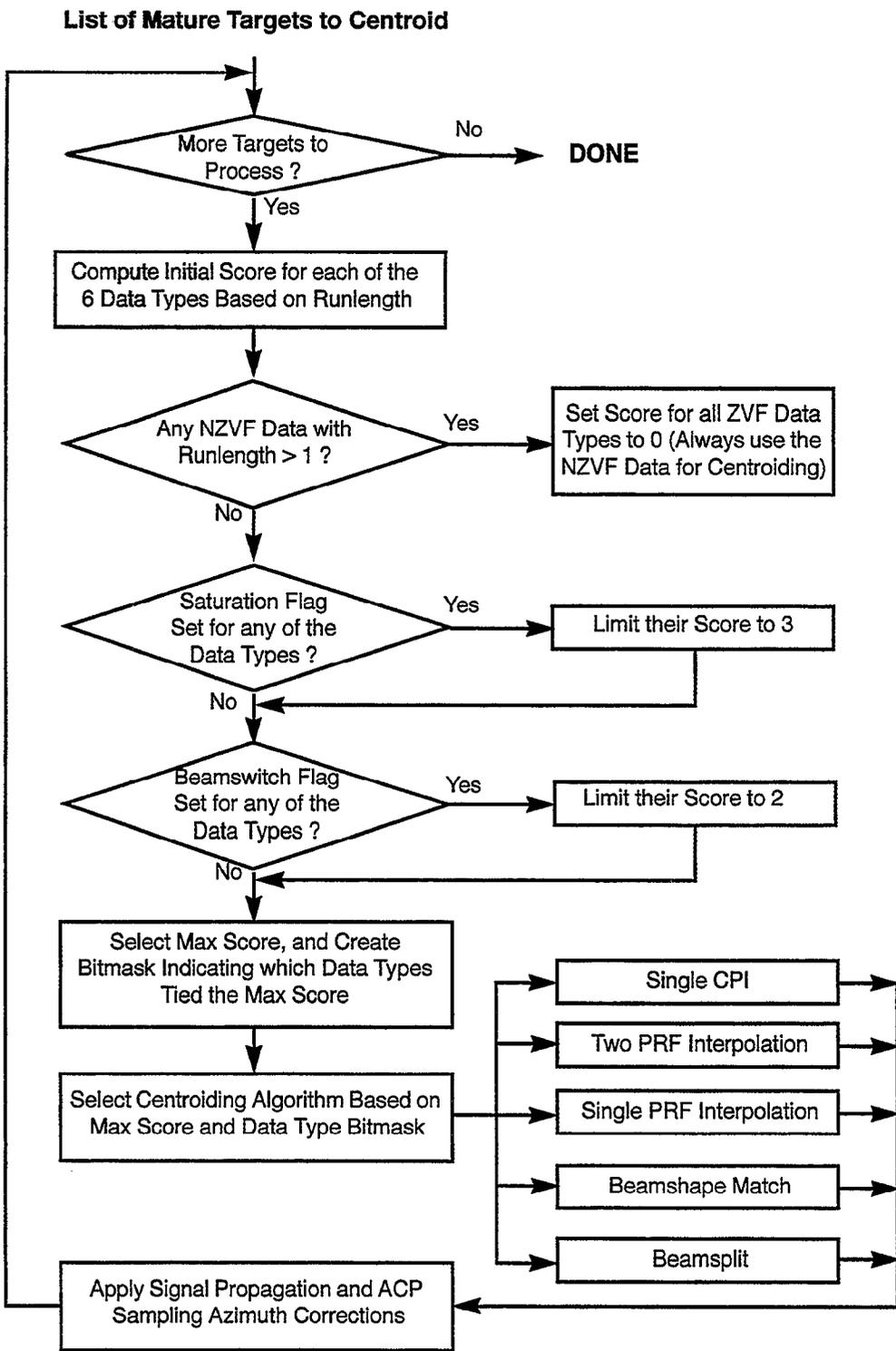
Figure 26. Azimuth centroiding.
