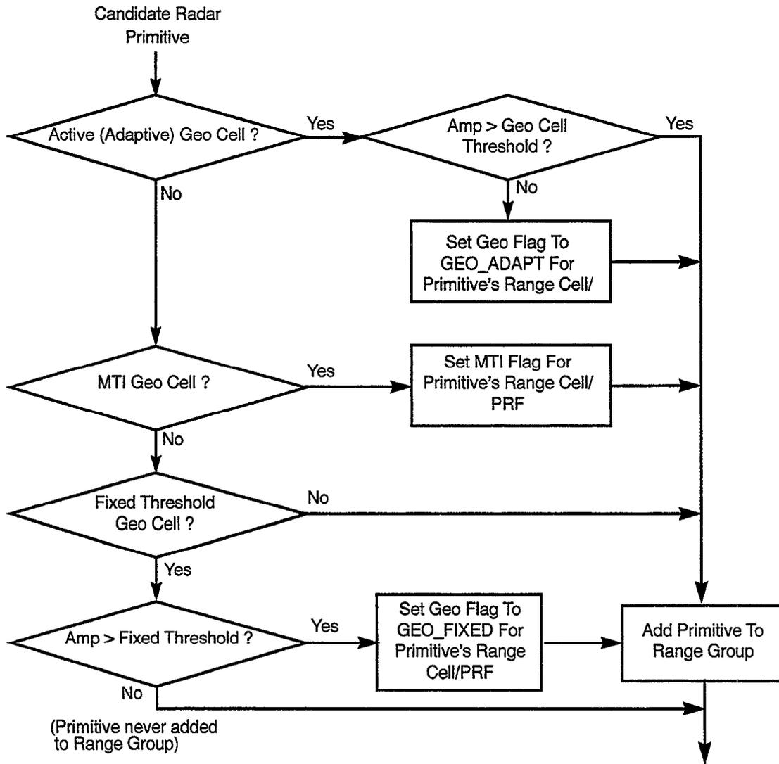
Figure 20. Front-end geocensor processing.
