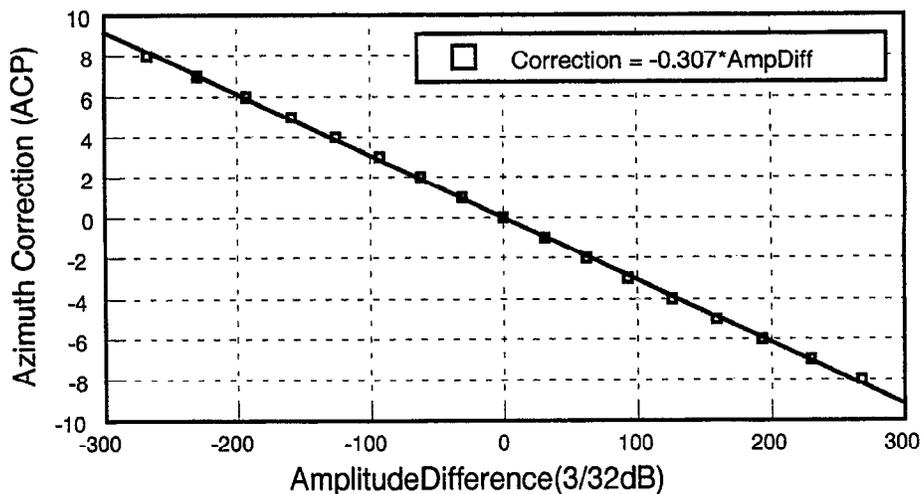
Figure 9. Azimuth correction vs. CPI amplitude difference.
