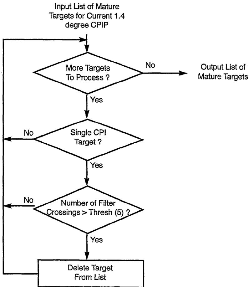
*Figure 25. Primary RFI processing.*
