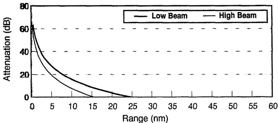
Figure 3. ASR-9 STC attenuation vs. range (typical).
