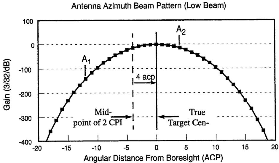
Figure 8. Antenna azimuth beam pattern (low beam).
