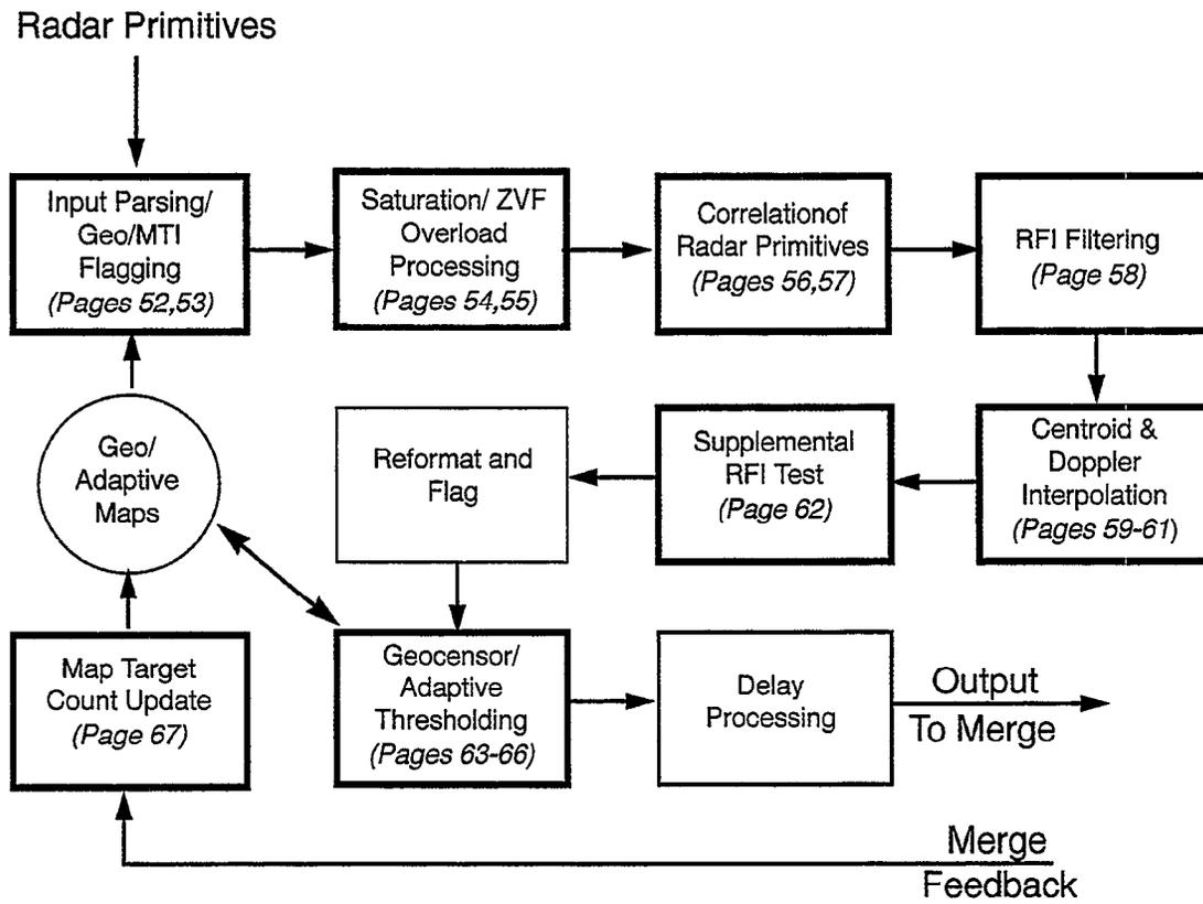
*Figure 18. C&I processing top level block diagram.*
