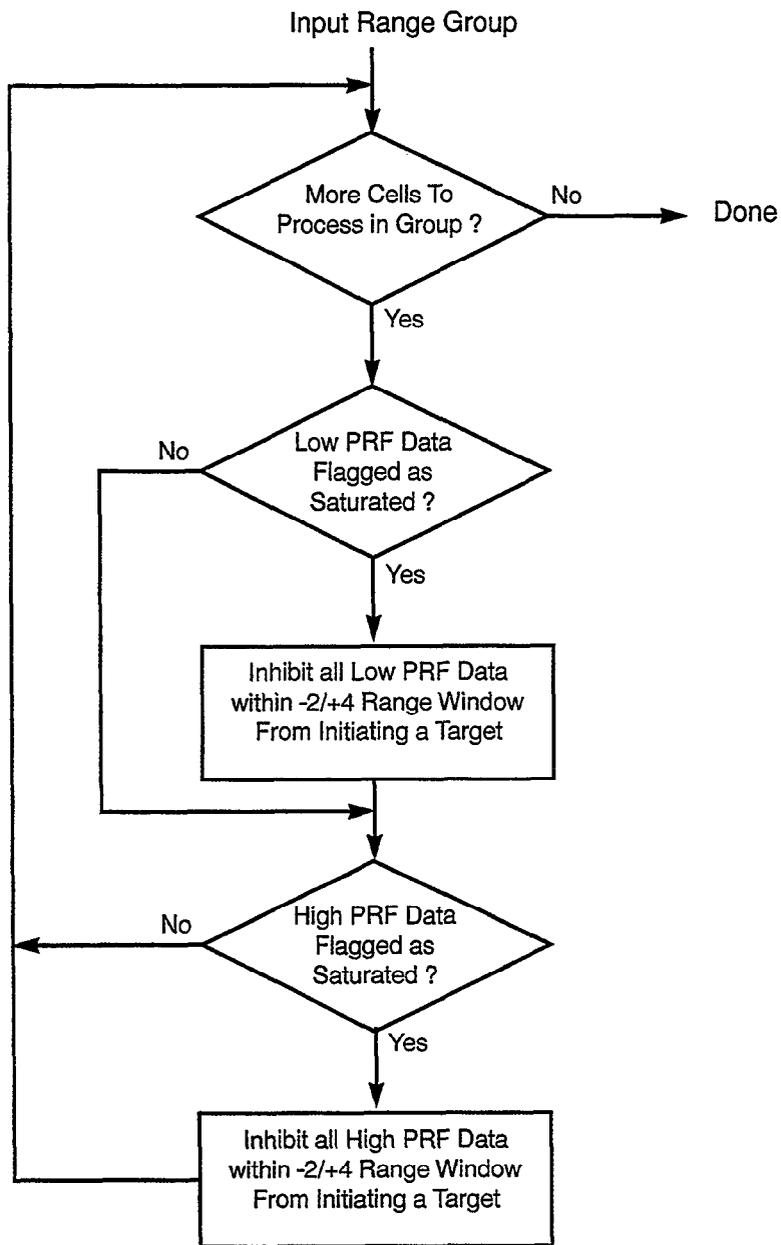
Figure 22. Saturation preprocessing.
