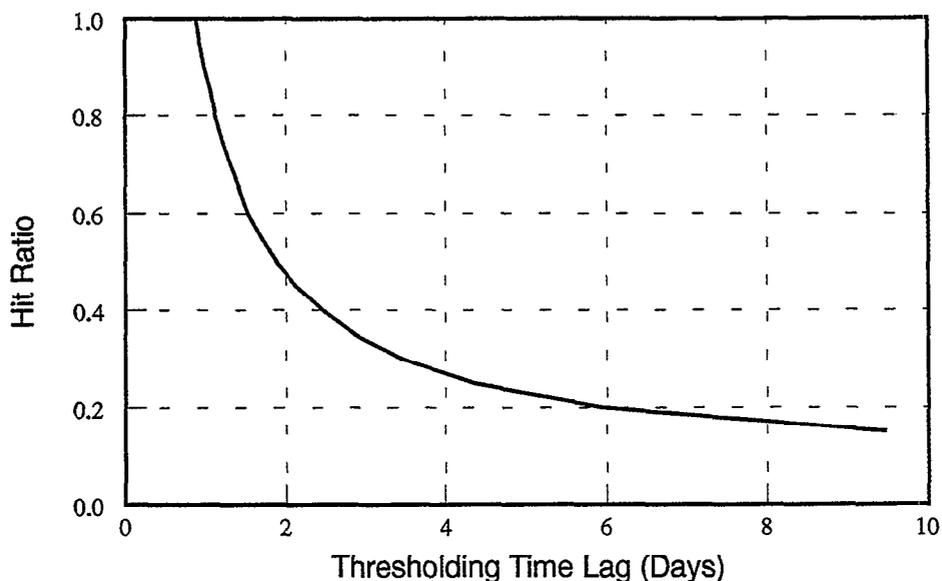
*Figure 14. Unmodified single pole filter thresholding time lag.*
