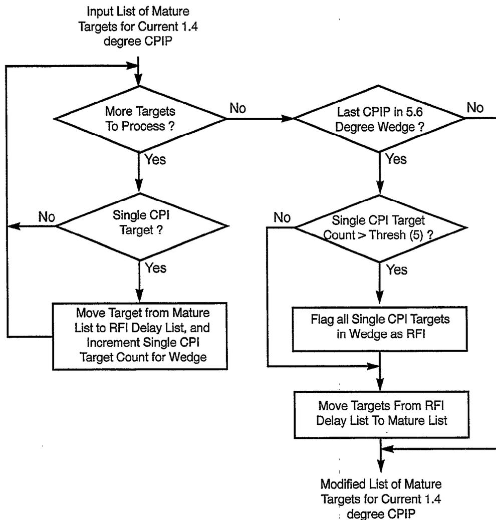
*Figure 29. Supplemental RFI processing.*
