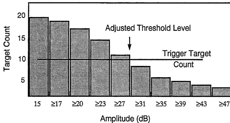
Figure 17. Adaptive map histogram-based threshold setting technique.
