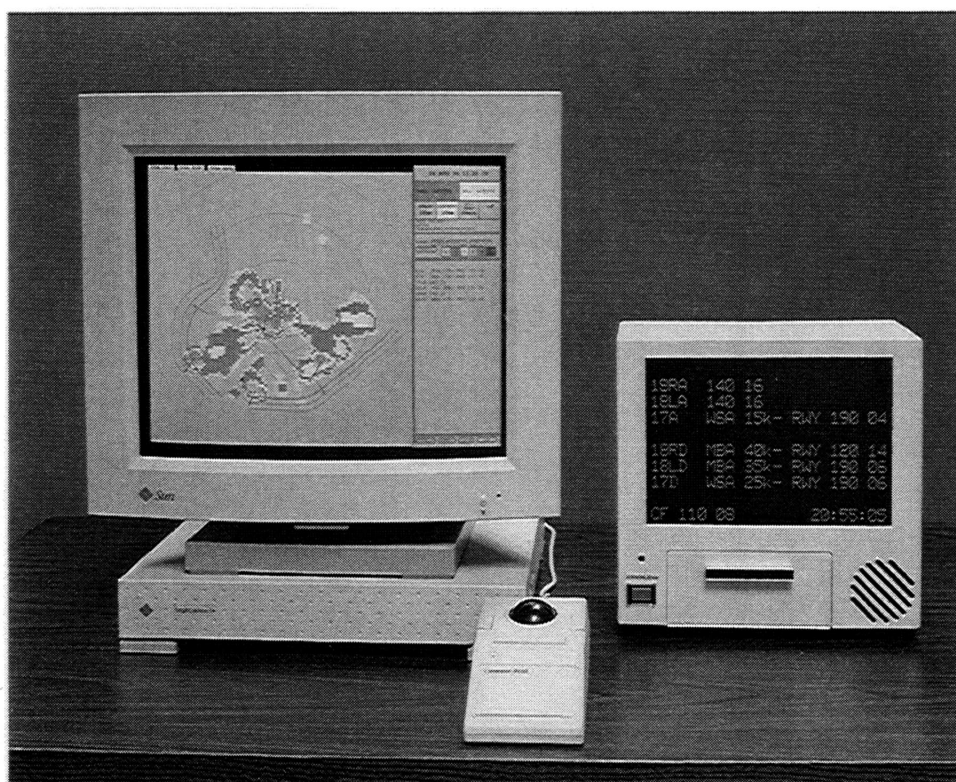
Figure 1. Supervisor's graphical situation display and local controller's ribbon display.
