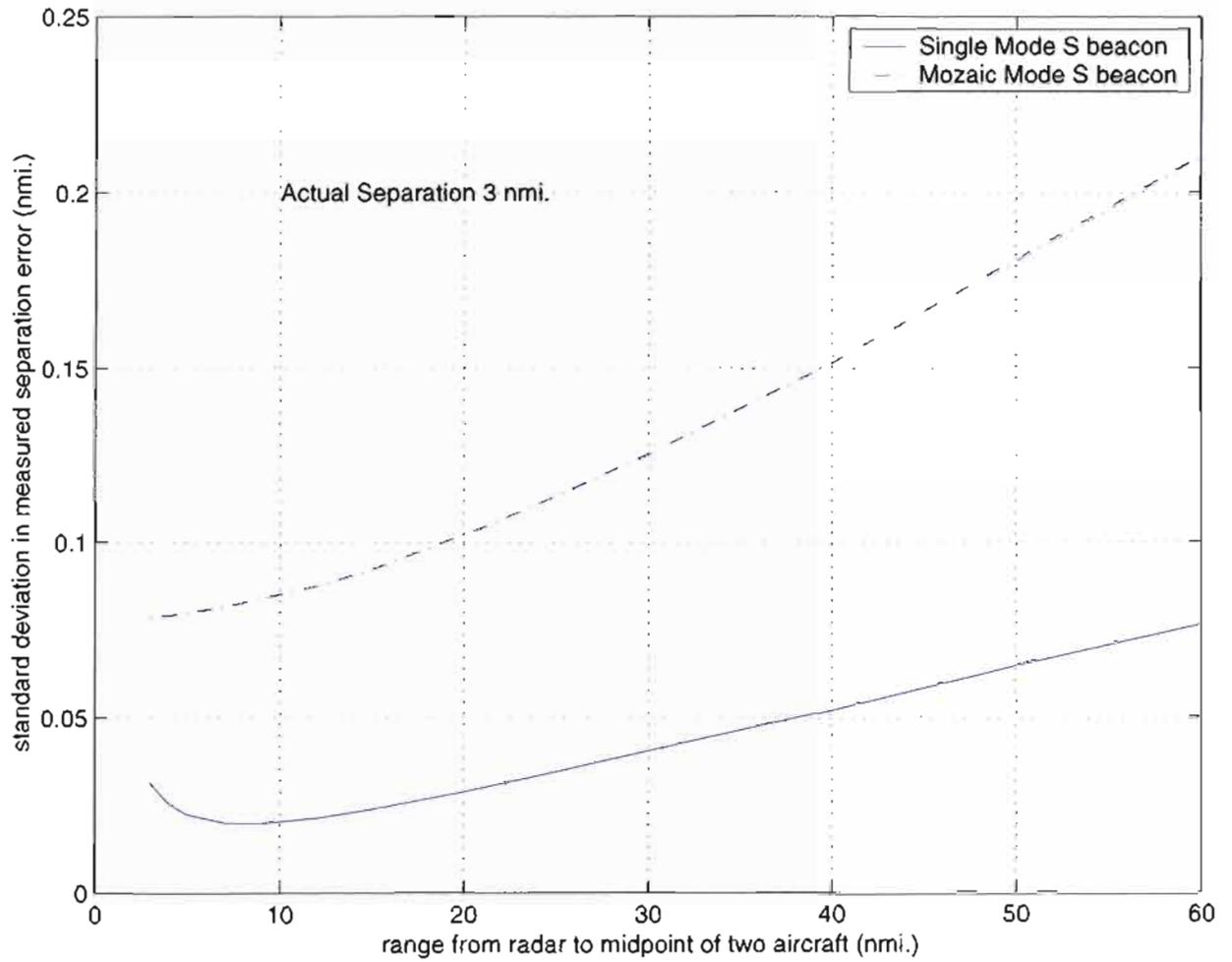
Figure 55. Standard deviation in measured separation error as a function of range for a single radar and for independent radars with a mosaic display. Range is the distance from the radar(s) to a point midway between two aircraft separated by 3 nautical miles as illustrated in Figure 4.
