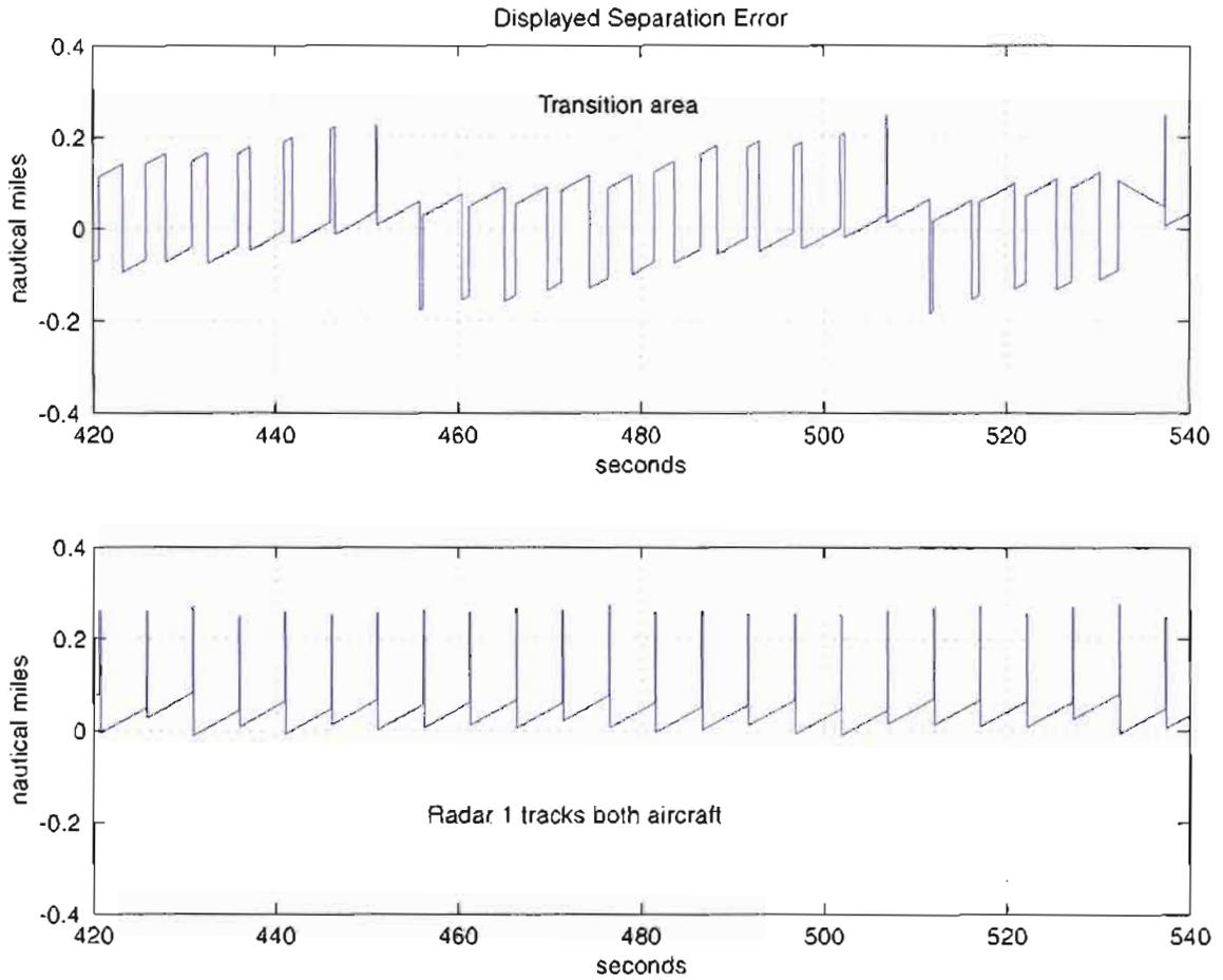
Figure 53. Displayed separation error as a function of time for specific case for radar 1 tracking both aircraft compared with radar 2 tracking until aircraft are within 15 nmi range of radar 1 – transition area
