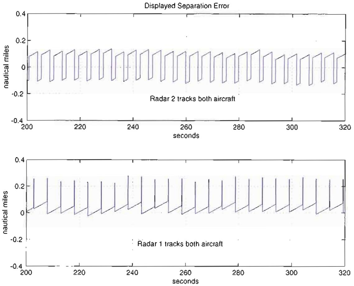
Figure 52. Displayed separation error as a function of time for specific case for radar 1 tracking both aircraft compared with radar 2 tracking until aircraft are within 15 nmi range of radar 1 – two minutes of initial tracking.
