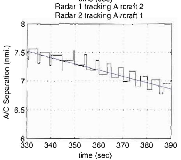
Figure 50. Displayed and actual separation as a function of time for a specific case for each combination of radar tracking aircraft, zoom-in of one minute during the middle of the track
