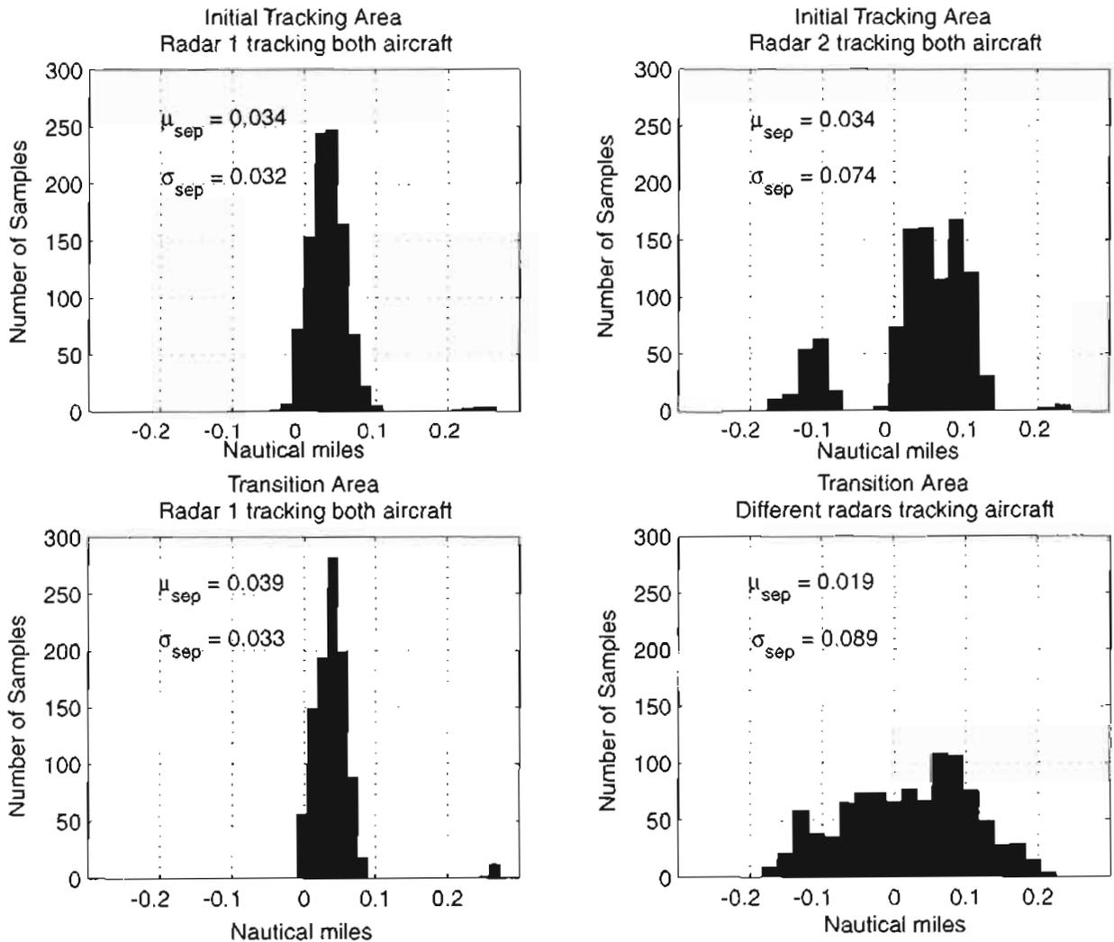
Figure 54. Histograms of displayed separation error in the initial tracking area and in the transition area for the cases where radar 1 tracked both aircraft and the cases where radar 2 tracked both aircraft in the initial tracking area and radar 1 tracked the aircraft within a 15 nmi range.
