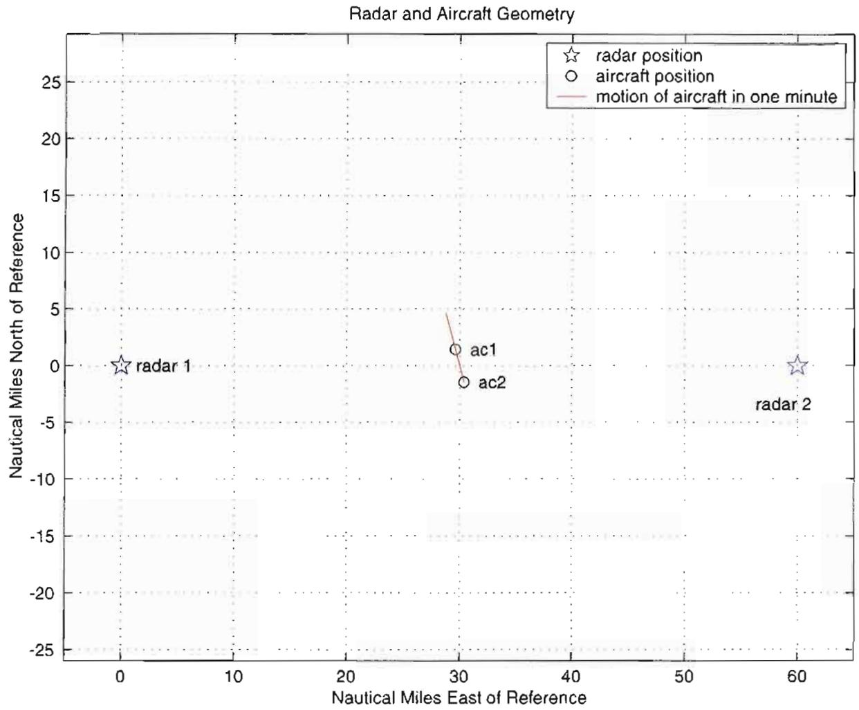
Figure 28. Radar and aircraft geometry for Case 2
