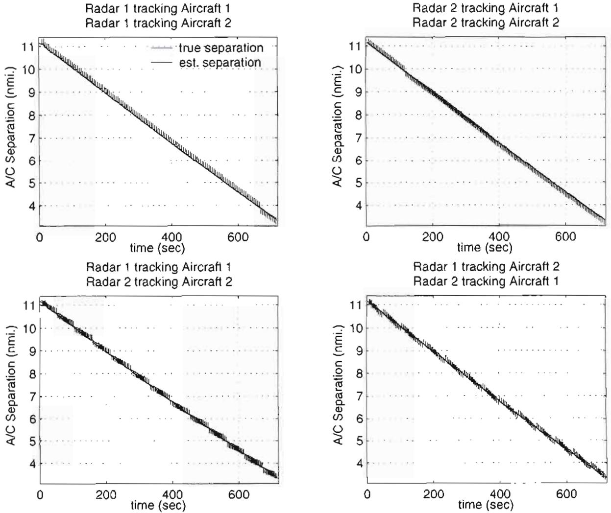
Figure 49. Displayed and actual separation as a function of time for a specific case for each combination of radar tracking aircraft
