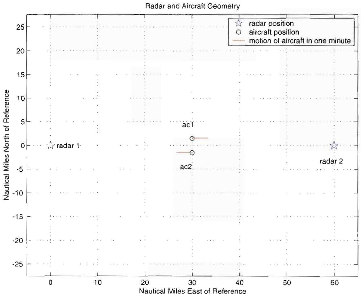
Figure 37. Radar and aircraft geometry for Case 4
