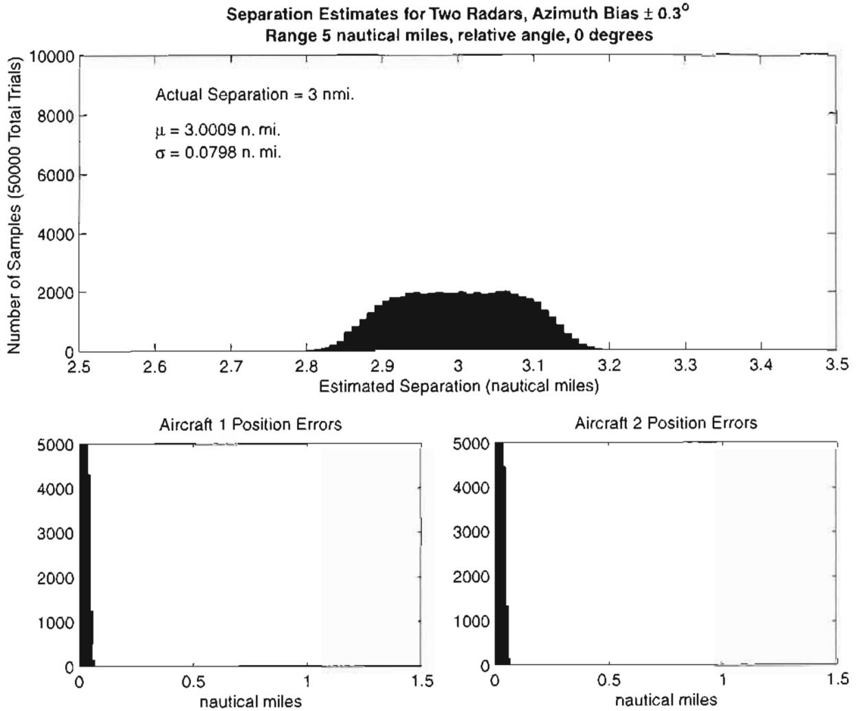
Figure 15. Average separation estimates for independent radars at 5 nmi Range.  $\Theta = 0'$
