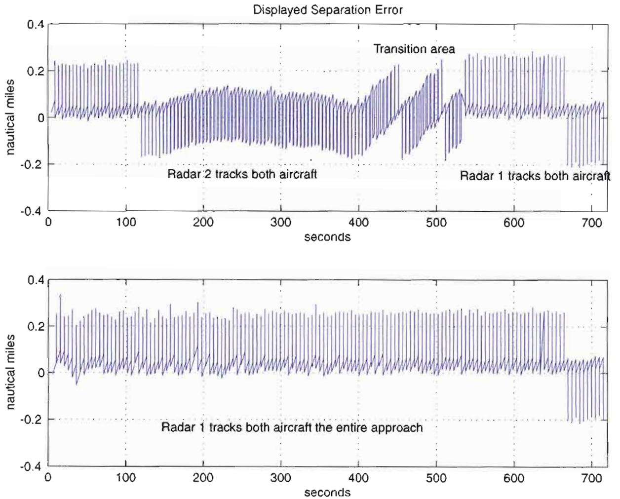
Figure 51. Displayed separation error as a function of time for specific case for radar 1 tracking both aircraft compared with radar 2 tracking until aircraft are within 15 nmi range of radar 1.
