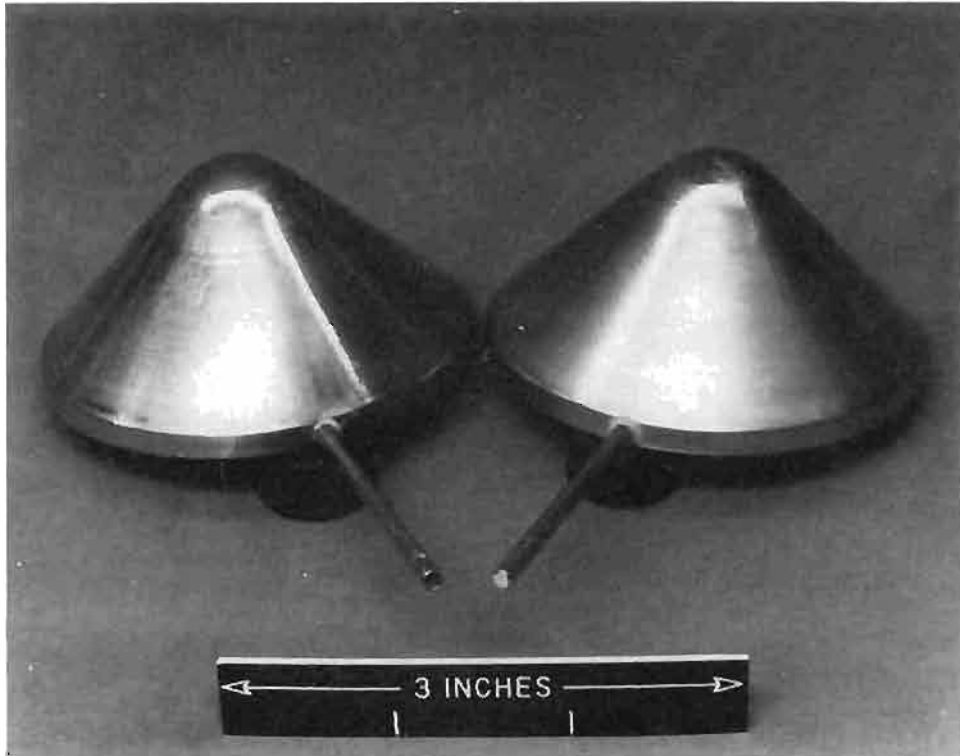
Figure III-3. Anemometer cup stems, by which the cups are held with set screws in the hub, are shown both before (left) and after (right) modification. Before, the hollow stem could be flattened as the cup was tightened in place; after, an aluminum plug prevents collapse of the stem.
