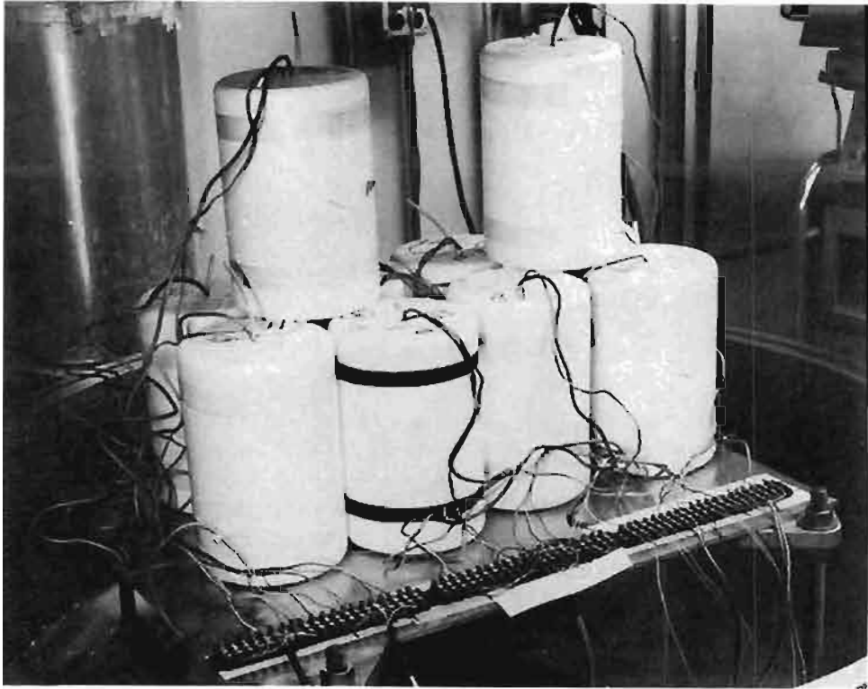
Figure III-14. View of 10 barometers mounted in pressure chamber just prior to testing. Visible are the styrofoam cylindrical containers providing the barometer thermal insulation. Tygon tubing input ports can be seen at the tops of the cylinders, next to wiring.
