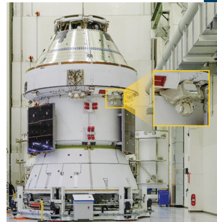
MAScOT is shown installed on the exterior of the Artemis II Orion spacecraft.
