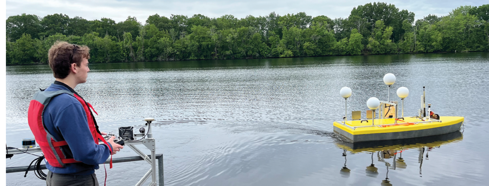
On the Merrimack River, Lincoln Laboratory intern and MIT student Robbie Khazan tests a prototype ASV equipped on the keel with a sonar array for sending and receiving acoustic signals, and above the surface with sensors for relative positioning.
