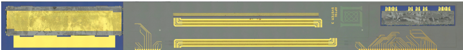
This photonic integrated circuit (measuring 3 x 0.5 cm) contains all the photonic components required for filtering and frequency down-converting millimeter-wave signals.
