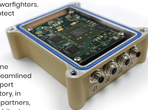
The SCM/ECU is packaged in a compact, tamper-protected box with data and control ports (J1–J4).
