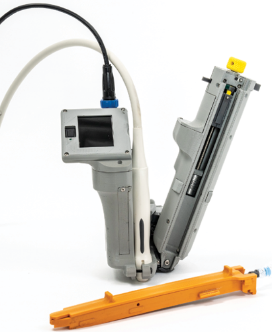
AI-GUIDE is a handheld device combining ultrasound, a user-guidance screen, blood-detecting optics, and a cartridge preloaded with a guide wire for accessing major blood vessels.
