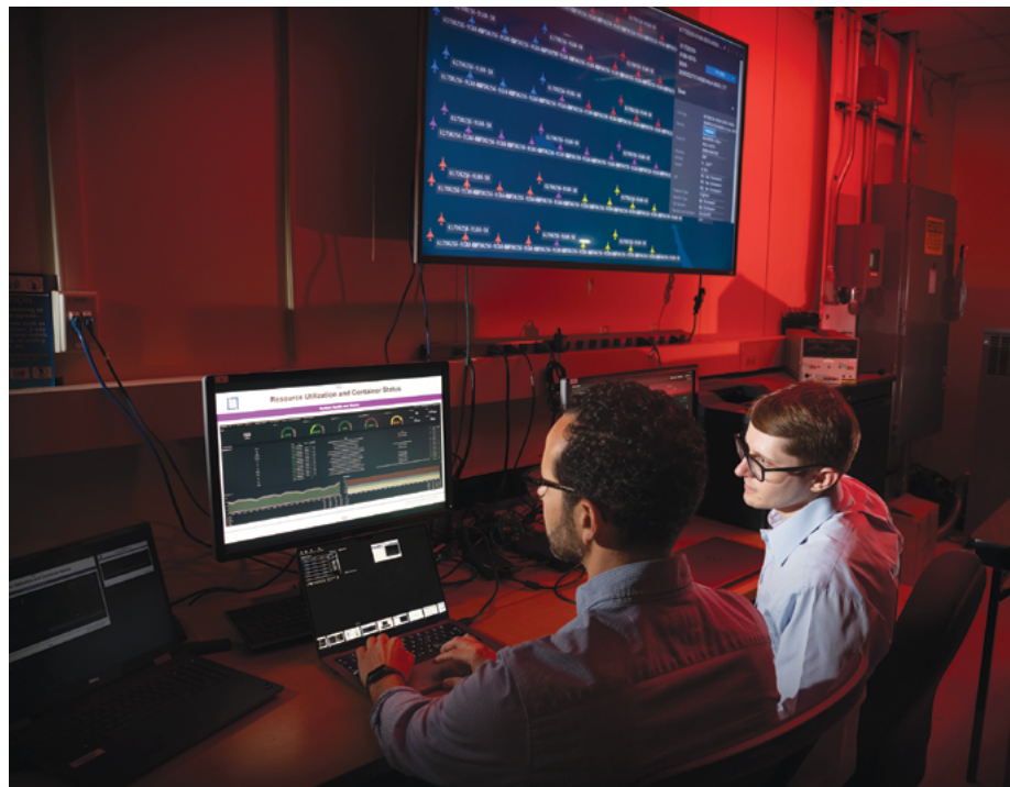
Scott Arbiv and Ted Richards monitor network performance as emulated traffic (airplane symbols) generated on an Air Force node is published to JTEN, where disadvantaged users subscribe to content based on geography or entity type (hostile or friendly).
